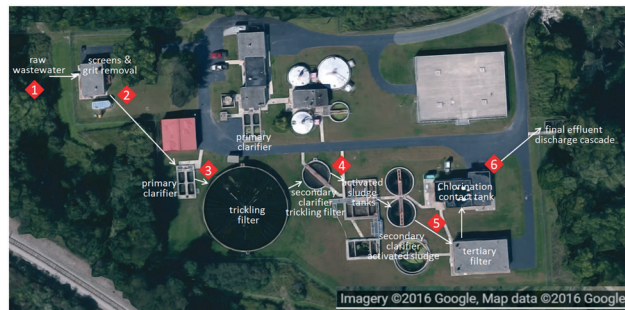
Fig. 2 Aerial view of Northfield WWTP with six sampling locations for the liquid stream: 1) raw wastewater, 2) preliminary effluent, 3) primary effluent, 4) secondary trickling filter, 5) secondary activated sludge system, and 6) final effluent.
