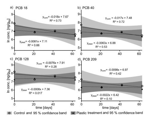
Fig. 2 Kinetic plots (natural log-transformed and lipid-normalized PCB concentrations over time) of the elimination rates of PCB 18 (a), PCB 40 (b), PCB 128 (c) and PCB 209 (d) in the control ("cont") and the plastic ("plast") treatment over a depuration time of 63 days.
