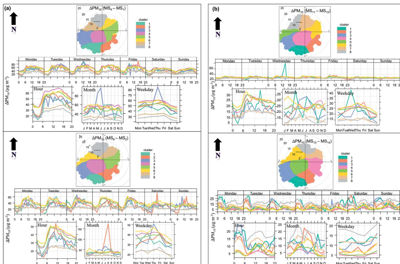
Fig. 5 Clusters identified at the CS<sub>1</sub> and CS<sub>2</sub> sites for  $PM_{10}$  concentrations for 8 clusters. The shading shows the 95% confidence intervals in the mean. The data have been normalised in each case by dividing by the mean.
