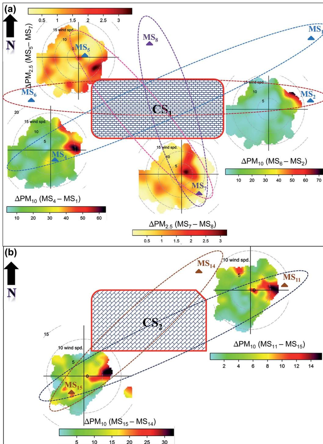
Fig. 4 The polar plots for the paired monitoring stations across each construction site, for  $\Delta\text{PM}_{10}$  and  $\Delta\text{PM}_{2.5}$  (a) at CS<sub>1</sub> and (b) for  $\Delta\text{PM}_{10}$  at CS<sub>2</sub>. These plots are presented as smoothed surfaces, showing that the concentrations vary depending on the local wind speed and wind direction.
