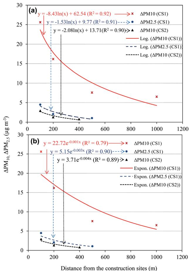
Fig. 9  $\Delta PM_{10}$  and  $\Delta PM_{2.5}$  concentration decay at CS<sub>1</sub> and CS<sub>2</sub> versus the distance in the direction of wind blowing from the construction sites showing the (a) logarithmic and (b) exponential best fit functions. In the fitting equations,  $x$  and  $y$  express the distance from principal construction site and the  $PM_{10}$  values, respectively. The solid lines represent the best fitting decay curves.
