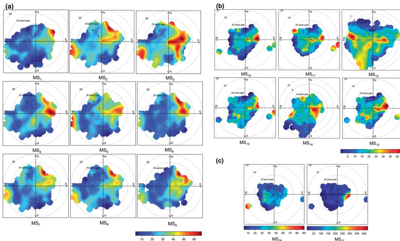
**Fig. 2** Polar plots for PM<sub>10</sub> at (a) CS<sub>1</sub>, (b) CS<sub>2</sub> and (c) CS<sub>3</sub>; hourly average values were used for all pollutants. These plots are presented as smoothed surfaces showing how the concentrations vary depending on the local wind speed and wind direction.
