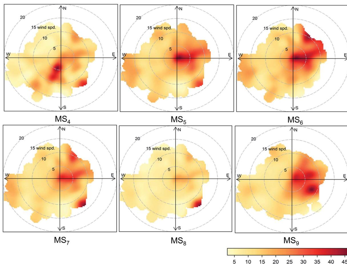
Fig. 3 Polar plots for  $PM_{2.5}$  (hourly average values were used for all pollutants) at  $CS_1$ . These plots are presented as smoothed surfaces showing how the concentrations vary depending on the local wind speed and wind direction.
