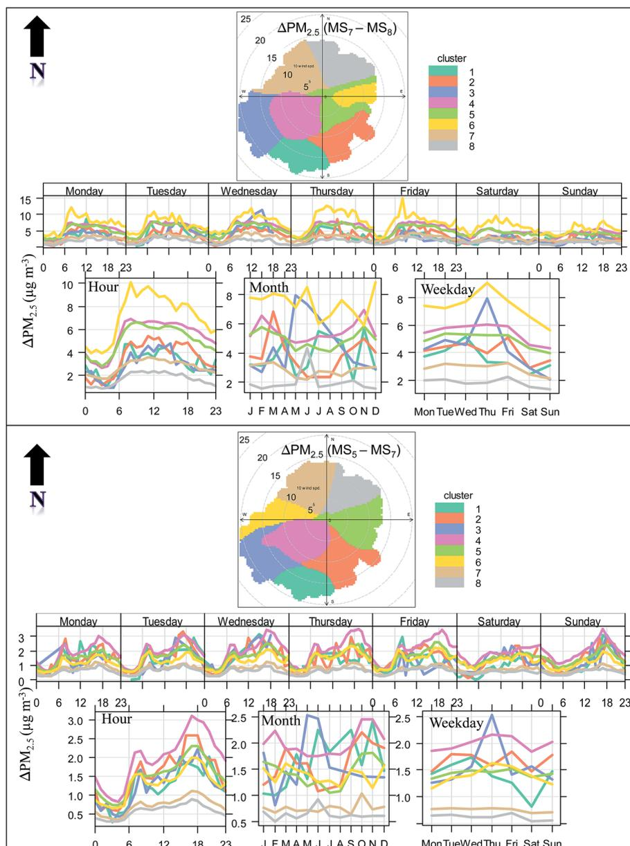
Fig. 6 Clusters identified at CS<sub>1</sub> for PM<sub>2.5</sub> concentrations for 8 clusters. The shading shows the 95% confidence intervals in the mean. The data have been normalised in each case by dividing by the mean.
