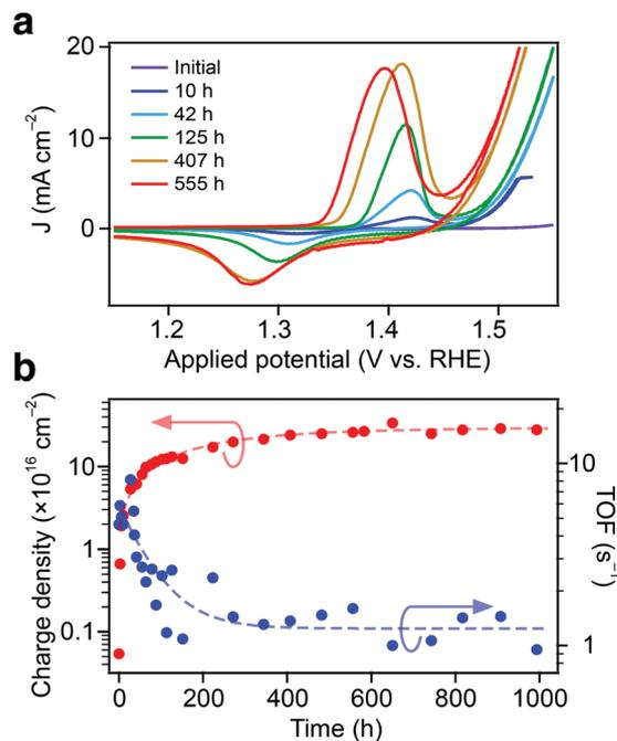
Fig. 2 (a) Examples of cyclic voltammograms of a Gibeon electrode measured at  $10 \text{ mV s}^{-1}$  after different oxidation periods in 1 M NaOH. (b) Charge density quantified under the reduction peak appearing in cyclic voltammograms and the turn-over frequencies (TOF) against operation time at  $500 \text{ mA cm}^{-2}$  (dotted lines: logistic function fits).
