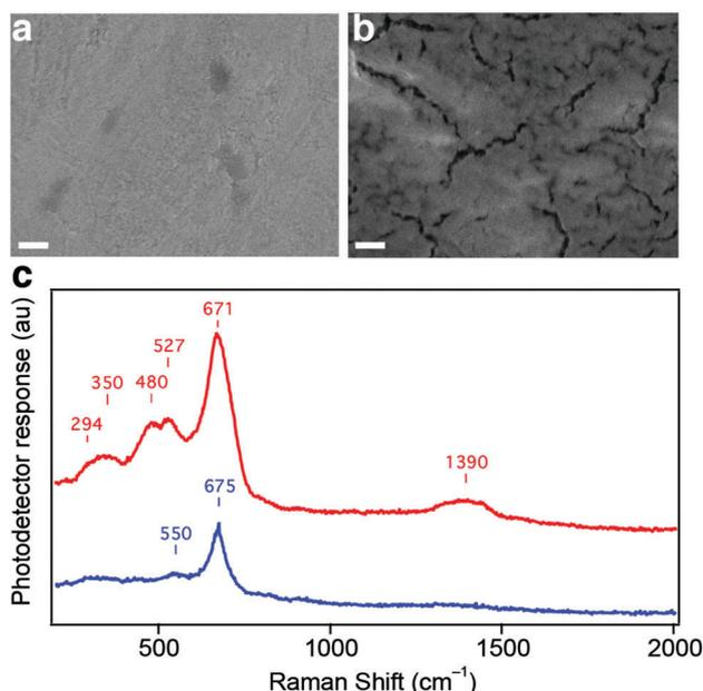
Fig. 3 Scanning electron micrographs of a Gibeon electrode before (a) and after (b) 50 hours of operation at 500  $\text{mA cm}^{-2}$  in 1 M NaOH (scale bars 200 nm) and (c) Raman spectra of a Gibeon sample before (blue) and after 48 hours of oxidation (red). Raman shift positions of the detected peaks are overlaid on the graph.
