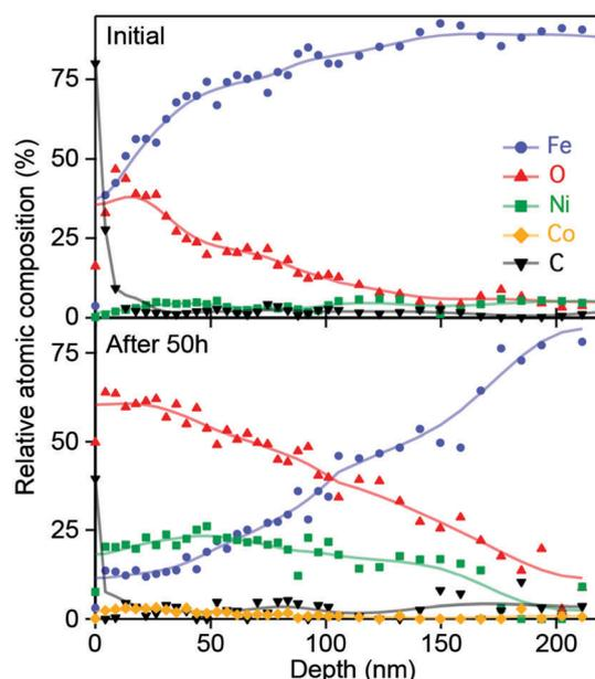
Fig. 4 Atomic composition profile obtained *via* XPS of a Gibeon sample before (top) and after 50 hours of operation at 500  $\text{mA cm}^{-2}$  in 1 M NaOH electrolyte (bottom). Spectra were obtained for both samples at different times after etching the surface with  $\text{Ar}^+$  ions at a rate of 8.8  $\text{nm min}^{-1}$ .
