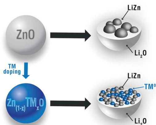
Fig. 8 Schematic illustration of the impact of introducing a TM dopant into ZnO on the lithiation mechanism and LiZn (Zn<sup>0</sup>) crystallite growth according to the findings of Mueller *et al.*<sup>48</sup>
