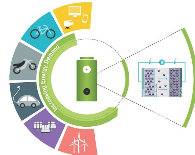
**Fig. 1** Schematic drawing of the general working principle (on the right) of lithium-ion batteries, with lithium cations shuttling from one electrode to the other accompanied by a unidirectional electron transfer along an outer circuit, and their current and foreseen applications (on the left), ranging from portable electronic devices to electrified transportation, including electric scooters and vehicles, as well as stationary energy storage for renewables.
