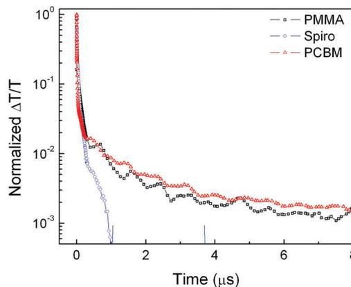
Fig. 3 Transient absorption decay probed at 750 nm for samples coated with PMMA, PCBM, and Spiro. The excitation wavelength was 532 nm at  $10^{18} \text{ cm}^{-3}$  initial excitation density. A zoomed in version of the long living tails is plotted on a linear scale in Fig. S5 (ESI<sup>†</sup>).
