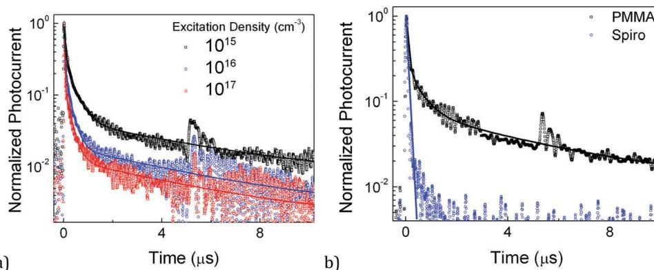
**Fig. 2** (a) Transient photocurrent (20 V) of a device upon 690 nm excitation at three different excitation densities. The device is covered with just an inert PMMA layer. (b) Transient photocurrent (20 V) traces for devices with the hole accepting Spiro and inert PMMA layers, measured at 690 nm at  $10^{15} \text{ cm}^{-3}$  excitation densities.
