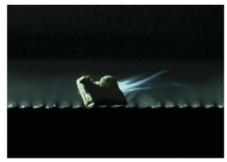
**Fig. 1** Self-propelled crystalline cellulose particle on an 800 °C microratcheted steel surface with back lighting. The vapor contrail extending from the particle results from motion of the solid particle from left to right.
