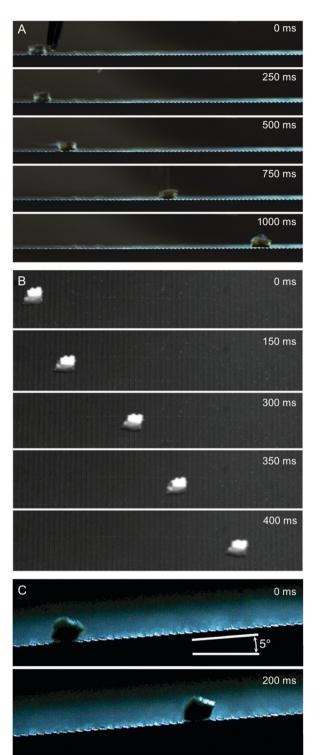
Fig. 3 Photography of self-propelled cellulose particles on 800 °C surface. (A) A particle of cellulose moves across a ratcheted surface viewed from a low angle  $(0-5^{\circ})$  with backlighting. (B) View from higher angle  $(\sim 45^{\circ})$  with front lighting. The ratchets are visible as dark, vertical stripes. (C) A particle of cellulose is propelled up the ratcheted surface inclined 5°. Image scale is provided by the visible ratchets.
