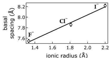
Fig. 5 Correlation of ionic radii<sup>52</sup> of intercalated halogen anions A<sup>m-</sup> with basal spacings of [NiFe]-(A<sup>m-</sup>)-LDH materials. Open circles, data; line, linear fit.
