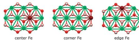
Fig. 12 Fe sites in the basic [Ni<sub>9</sub>Fe<sub>1</sub>(OH)<sub>18</sub>]<sup>3+</sup> cluster fragment. Colors: Ni green, Fe maroon, O red, H white.
