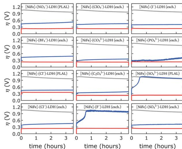
**Fig. 9** Constant current electrolysis of [NiFe]-LDH materials with different interlayer anions in virtually carbonate-free electrolyte in a glove box (blue) and in 1.0 M aqueous KOH in ambient air (red). Chronopotentiometry data of bare HOPG are shown in grey. All data were collected at a constant current density of 1 mA cm<sup>-2</sup>.
