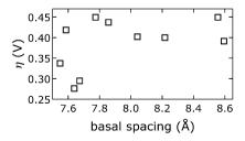
Fig. 11 Observed overpotentials  $\eta$  at 10 min from chronopotentiometry data collected in virtually carbonate-free electrolyte (glove box) as a function of the basal spacing of [NiFe]-LDH materials with different interlayer anions.
