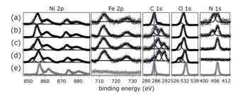
Fig. 2 XPS data of [NiFe]–(NO $_3$ <sup>-</sup>)-LDH (as synthesized, a) and exchanged in different pH aqueous KOH solutions (b, pH 8.0; c, pH 11.0; d, pH 14.0). Depicted in grey are data of commercial Ni(NO $_3$ )<sub>2</sub>-6H<sub>2</sub>O (e). The blue line in the C 1s panel indicates the binding energy of adventitious carbon. Open circles, data; lines, peak fits.
