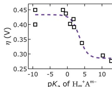
**Fig. 10** Overpotentials  $\eta$  of [NiFe]-LDH materials with different interlayer anions A<sup>m-</sup> derived from constant current electrolysis at 1 mA cm<sup>-2</sup> in virtually carbonate-free electrolyte as a function of anion basicity. Open squares, data; dashed line, sigmoidal fit.
