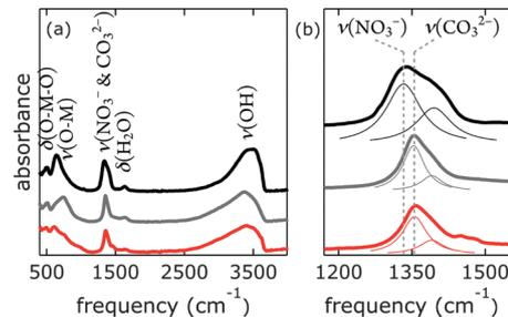
Fig. 6 Infrared spectra of [NiFe]-(NO<sub>3</sub><sup>-</sup>)-LDH nanosheets as synthesized (black), after being suspended in 0.1 M aqueous K<sub>2</sub>CO<sub>3</sub> solution (grey), and after being suspended in 0.1 M aqueous KOH (red); (a) full spectra, (b) magnification of the region characteristic for NO<sub>3</sub><sup>-</sup> and CO<sub>3</sub><sup>2-</sup>, Lorentzian fits are depicted as thin lines.
