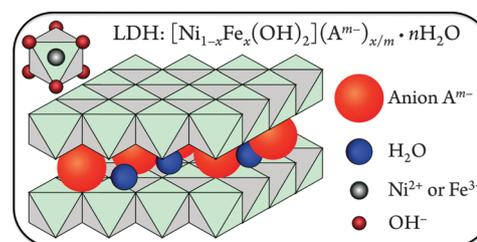
Fig. 1 Schematic illustration of the [NiFe]-LDH structure. Anions and water are present in the interlayer space, and  $\text{Ni}^{2+}$  or  $\text{Fe}^{3+}$  ions are surrounded by six hydroxides in distorted octahedral coordination (upper left).
