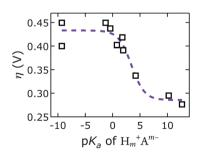
Fig. 10 Overpotentials  $\eta$  of [NiFe]-LDH materials with different interlayer anions  $A^{m-}$  derived from constant current electrolysis at 1 mA cm $^{-2}$  in virtually carbonate-free electrolyte as a function of anion basicity. Open squares, data; dashed line, sigmoidal fit.
