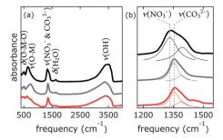
Fig. 6 Infrared spectra of [NiFe]-(NO<sub>x</sub>-)-LDH nanosheets as synthesized (black), after being suspended in 0.1 M aqueous K<sub>2</sub>CO<sub>3</sub> solution (grey), and after being suspended in 0.1 M aqueous KOH (red); (a) full spectra, (b) magnification of the region characteristic for NO<sub>3</sub><sup>-</sup> and CO<sub>3</sub><sup>2-</sup>, Lorentzian fits are depicted as thin lines
