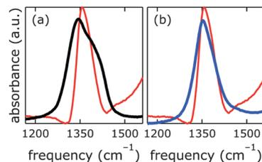
Fig. 7 Infrared spectra of [NiFe]-(NO<sub>3</sub><sup>-</sup>)-LDH nanosheets as synthesized (black), after being suspended in carbonate-free strong base electrolyte in Ar atmosphere as described above (blue), and after being suspended in 0.1 M aqueous KOH in ambient air (red).
