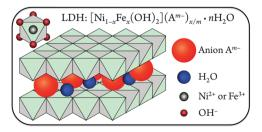
Fig. 1 Schematic illustration of the [NiFe]-LDH structure. Anions and water are present in the interlayer space, and  $\mathrm{Ni}^{2+}$  or  $\mathrm{Fe}^{3+}$  ions are surrounded by six hydroxides in distorted octahedral coordination (upper left).
