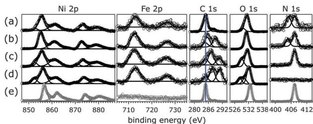
Fig. 2 XPS data of [NiFe]-(NO<sub>3</sub><sup>-</sup>)-LDH (as synthesized, a) and exchanged in different pH aqueous KOH solutions (b, pH 8.0; c, pH 11.0; d, pH 14.0). Depicted in grey are data of commercial Ni(NO<sub>3</sub>)<sub>2</sub>·6H<sub>2</sub>O (e). The blue line in the C 1s panel indicates the binding energy of adventitious carbon. Open circles, data; lines, peak fits.
