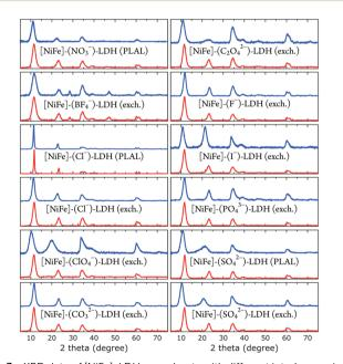
Fig. 3  $\,$  XRD data of [NiFe]-LDH nanosheets with different interlayer anions as synthesized (blue) and after suspension in 1.0 M aqueous KOH in ambient air (red).
