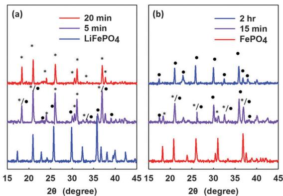
Fig. 3 XRD patterns of LiFePO<sub>4</sub>/FePO<sub>4</sub> at different time intervals of chemical (a) delithiation and (b) lithiation. \* represents the peaks of FePO<sub>4</sub> and ● represents the peaks of LiFePO<sub>4</sub>.
