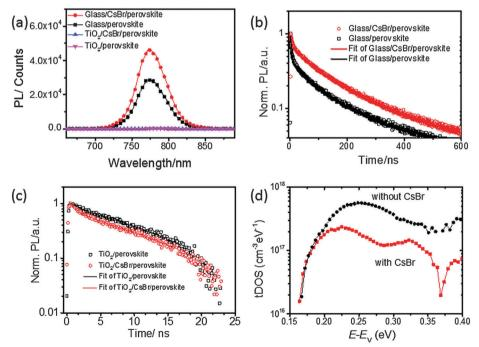
Fig. 3 (a) Steady-state photoluminescence spectra of perovskite thin films deposited on glass and c-TiO2 layer with and without CsBr modification collected following excitation at 510 nm, (b) time-resolved photoluminescence spectra of perovskite thin films on glass collected at 400 kHz (c) and on c-TiO<sub>2</sub> layer collected at 30 MHz at 0.03 μJ per cm<sup>2</sup> per pulse, (d) trap density of states (tDOS) for devices without CsBr (black) and with CsBr modification (red)
