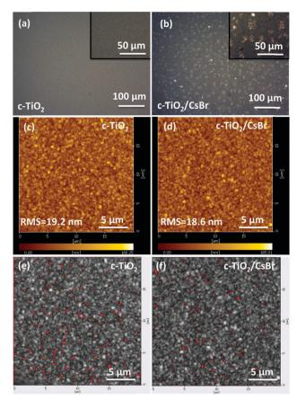
Fig. 1 Microphotographs of (a) TiO<sub>2</sub> compact layer (c-TiO<sub>2</sub>) and (b) c-TiO<sub>2</sub>/ CsBr substrates after coloration. AFM topography of a c-TiO<sub>2</sub> on FTO glass without (c) and with (d) CsBr modification; (e) and (f) show the corresponding height mapping.
