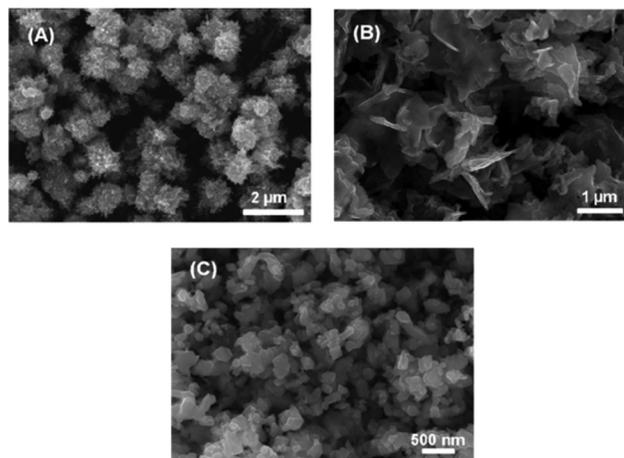
Fig. 7 SEM images of  $\text{Fe}_3\text{Se}_4$  (a) 'nanocacti', (b) nanosheets, and (c) nanoplatelets synthesized by Zhang *et al.*,<sup>79</sup> with the morphology dictated by the amount of oleic acid present in the reaction. Reprinted with permission from ref. 79, ©2011 American Chemical Society.
