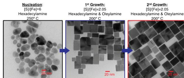
Fig. 2 TEM images and conditions employed by Macpherson *et al.*<sup>2</sup> during their synthesis of pyrite nanocubes. Reprinted with permission from ref. 2, ©2012 American Chemical Society.
