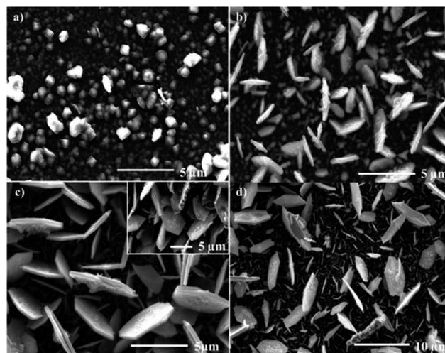
**Fig. 5** SEM images of troilite thin films produced from the aerosol assisted chemical vapour deposition of  $[\text{Fe}(\text{SON}(\text{CNEt}_2)_2)_3]$  at (a) 300 °C, (b) 350 °C, (c) 400 °C (inset 45° tilt image of film) and (d) 450 °C. Reprinted with permission from ref. 68, ©2010 American Chemical Society.
