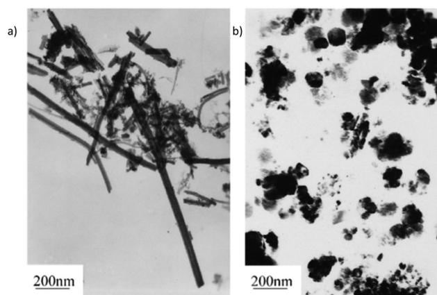
Fig. 4 The solvothermal reaction of  $\text{FeSO}_4 \cdot 7\text{H}_2\text{O}$  and  $\text{Na}_2\text{S}_3$  gives nanorods in ethylenediamine and nanoparticles in benzene, demonstrating the solvent dependency of the morphology. Reprinted with permission from ref. 38, ©2001 Elsevier.
