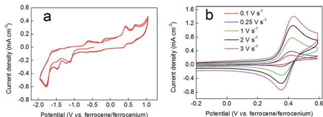
**Fig. 9** Cyclic voltammograms of an 11 mM solution of the nitrate salt of complex **3** in 0.5 M TBA-PF<sub>6</sub>/acetonitrile obtained under the conditions detailed in the Experimental section (with the exception that a Pt counter electrode was used). (a) A full range cyclic voltammogram at a scan rate of 0.1 V s<sup>-1</sup>. (b) CVs as in panel (a), but at various scan rates as indicated. The ferrocene/ferrocenium couple is not shown for clarity.
