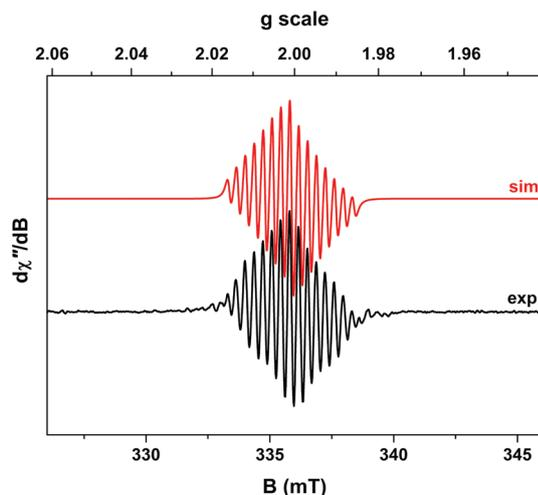
**Fig. 3** X-band EPR spectrum of paramagnetic species generated from the reaction of complex **2** with  $\text{NOBF}_4$ , recorded in acetonitrile solution at 293 K (experimental conditions: frequency, 9.4053 GHz; power, 9.5 mW; modulation, 0.1 mT). Experimental data are represented by the black line and a simulation is depicted by the red trace.
