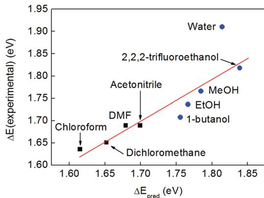
**Fig. 7** A plot of the experimental excitation energies against the predictions from a linear model incorporating the Onsager function  $f_{\text{O}}(\epsilon)$  and the Kamlet–Taft  $\alpha$ -parameter for hydrogen bond donor strength (taken from ref. 56). The linear fit function is  $\Delta E_{\text{pred}} = 1.345 \text{ eV} + 0.695 f_{\text{O}}(\epsilon) + 0.109 \alpha$ . Non-hydrogen bonding solvents are depicted with black squares, hydrogen bonding solvents with blue circles.
