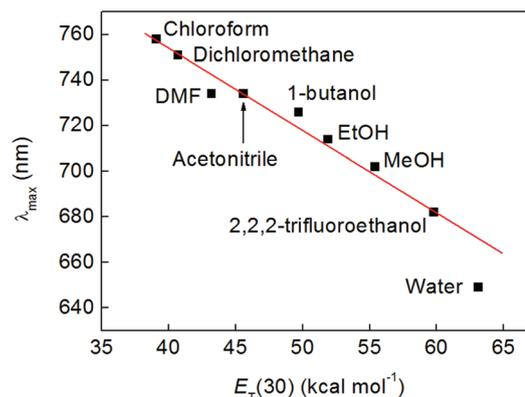
**Fig. 4** Wavelength of the lowest energy absorption band of compound **2** as a function of solvent polarity, plotted on the Dimroth–Reichardt  $E_{\text{T}}$  scale. All solutions were at a concentration of 5 mM, except those in butanol, chloroform and dichloromethane (2.5 mM). The red line is a linear fit and is provided as a guide to the eye.
