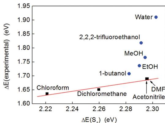
**Fig. 5** A plot of the experimental excitation energies (obtained from the band maxima given in Fig. 4) and the energies of the lowest excited singlet state calculated by TD-DFT ( $\omega$ B97-XD/def2-TZVP/PCM). Non-hydrogen bonding solvents are depicted with black squares and the linear trend is indicated by a red line as a guide to the eye. Hydrogen bonding solvents are shown as blue circles.
