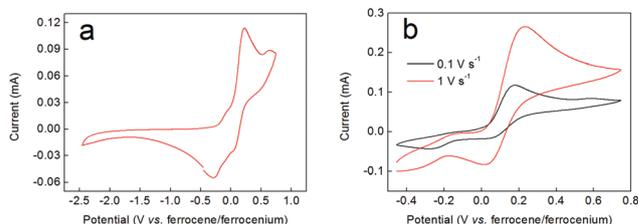
**Fig. 2** (a) Cyclic voltammogram of a 12 mM solution of the nitrate salt of complex **2** in 0.1 M TBA-PF<sub>6</sub>/acetonitrile run under the conditions detailed in the Experimental section. (b) Cyclic voltammograms as in panel (a), but over a narrower potential range and showing the effect of variation in the scan rate as indicated. The ferrocene/ferrocenium couple is not shown for clarity.
