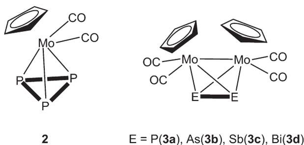
**Scheme 2** Representation of the tetrahedrane complexes  $[\text{CpMo}(\text{CO})_2(\eta^3\text{-P}_3)]$  (**2**) and  $[(\text{CpMo}(\text{CO})_2)_2(\mu, \eta^2: \eta^2\text{-E}_2)]$  (E = P(**3a**), As(**3b**), Sb(**3c**), Bi(**3d**)).
