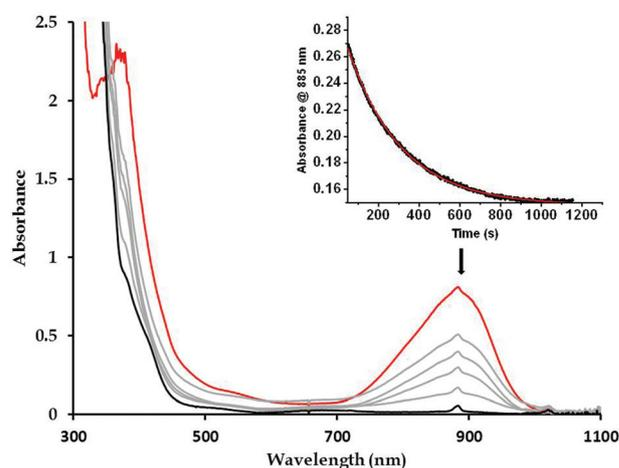
Fig. 5 Spectral changes of **3a** in the presence of 50 mM CCA at  $-60$  °C. Inset: Time trace of the decay at 885 nm band upon addition of the substrate (black trace) and the first-order fit (inset: red trace).
