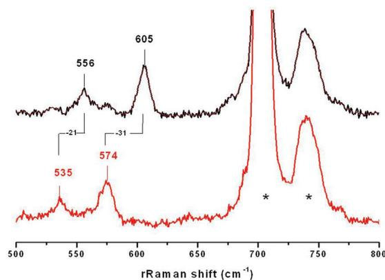
Fig. 3 Raman shifts obtained using a 413 excitation laser for **3a** involving <sup>16</sup>O (top) and <sup>18</sup>O (bottom) atoms. Bands originated from the solvent are marked by asterisks.
