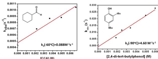
Fig. 6 Pseudo first-order rate constants as a function of substrate concentration; the reaction of **3a** with cyclohexane carboxaldehyde (left) and 2,4 di-*tert*-butylphenol (right) in CH<sub>2</sub>Cl<sub>2</sub>.
