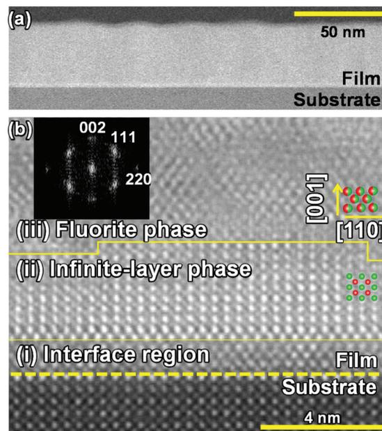
Fig. 2 (a) Wide and (b) magnified view of HAADF-STEM images after the reaction at 240 °C for 12 h. Inset: Fourier transform of the fluorite phase region (iii). Green and red circles show the positions of neodymium and nickel atoms, respectively.
