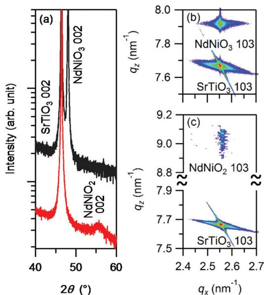
Fig. 1 (a) XRD  $2\theta$ - $\theta$  patterns before (black) and after (red) the reaction with CaH<sub>2</sub> at 240 °C. Reciprocal space maps (b) before and (c) after the reaction.
