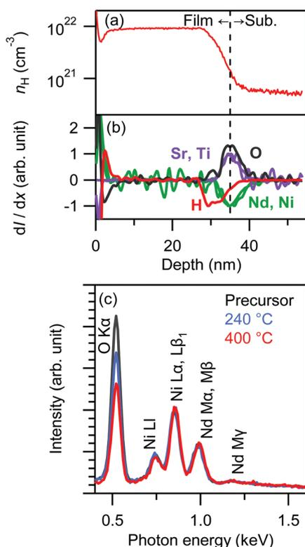
**Fig. 3** (a) Depth dependence of atomic hydrogen density ( $n_{\text{H}}$ ) after the reaction at 240 °C. (b) Differential secondary-ion intensity ( $dI/dx$ ) of each element. (c) EDS spectra of the films before (black) and after the reaction (blue, red), measured at an acceleration voltage of 2.5 kV.
