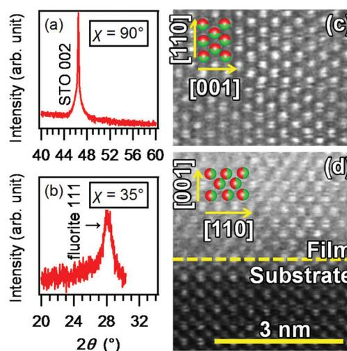
**Fig. 4** (a) Out-of-plane ( $\chi = 90^\circ$ ) and (b) asymmetric ( $\chi = 35^\circ$ ) XRD patterns of the films reacted at 400 °C for 24 h. HAADF-STEM images of the film reacted at 400 °C for 24 h (c) at the middle of the film and (d) at the interface between the film and the substrate.
