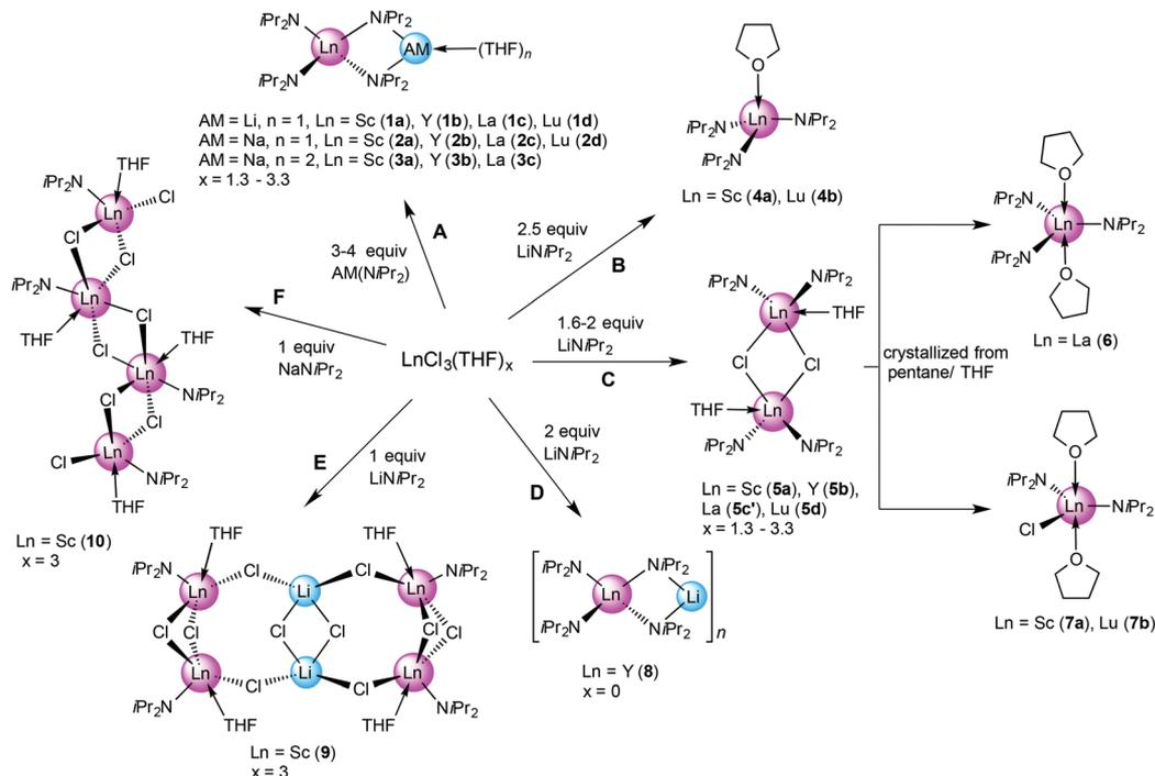
**Scheme 1** Overview of the syntheses of rare-earth metal diisopropylamide complexes *via* salt metathesis in *n*-hexane. The crystal structure of **5c'** shows a 1 : 1 mixture of dimeric **5c** and **6** in the asymmetric unit. The side products LiCl and NaCl were omitted for clarity.
