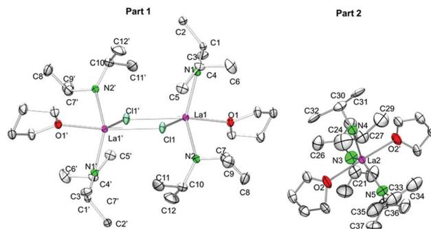
**Fig. 6** Crystal structure of [La(NiPr<sub>2</sub>)<sub>2</sub>(THF)(μ-Cl)]<sub>2</sub>·La(NiPr<sub>2</sub>)<sub>3</sub>(THF)<sub>2</sub> (5c'). Non-hydrogen atoms are represented by atomic displacement ellipsoids at the 30% level. Hydrogen atoms are omitted for clarity. The monomer (part 2) is heavily disordered and a partial disordering model is shown in the ESI (Fig. S11‡). For selected bond lengths and angles of part 1, see Table 3.
