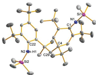
**Fig. 1** ORTEP drawing of the molecular structure of **8**. Thermal ellipsoids with 50% probability at 173 K (hydrogen atoms omitted for clarity except from N–H). Selected distances (Å) and angles (°): Si1–N1 1.689(2), Si2–N2 1.732(2), N1–C1 1.268(2), N2–C22 1.438(2), C29–C4 1.565(3), Si1–N1–C1 175.9(2), N2–Si2–C22 135.2(2).
