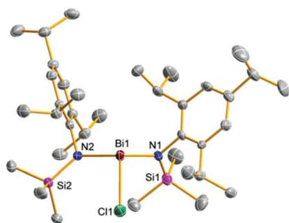
**Fig. 4** ORTEP drawing of the molecular structure of **9b**. Thermal ellipsoids with 50% probability at 173 K (hydrogen atoms omitted for clarity). Selected distances (Å) and angles ( $^\circ$ ): Bi1–Cl1 2.4862(7), Bi1–N1 2.140(2), Bi1–N2 2.179(2), N1–Bi1–Cl1 97.35(5), Cl1–Bi1–N2 95.83(5), N2–Bi1–N1 108.50(7).
