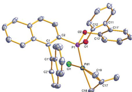
**Fig. 3** Molecular structure of (*S*)-**6a**. Hydrogen atoms have been omitted for clarity. Selected average bond distances (Å) and angles (°): Pd1–P1 2.2478(10), Pd1–C11 2.3583(9), Pd1–C17 2.162(4), Pd1–C18 2.195(4), Pd1–C19 2.096(4), P1–C2 1.815(4), P1–O1 1.619(3), P1–O2 1.610(3), C11–C11' 1.477(5); P1–Pd1–C11 91.55(4), P1–Pd1–C18 165.51(11), P1–Pd1–C19 98.27(13), C18–Pd1–C19 67.46(16), C18–C17–C19 114.6(4), C2–C1–C1'–C2' –80.8(5), C12–C11–C11'–C12' 42.3(6).
