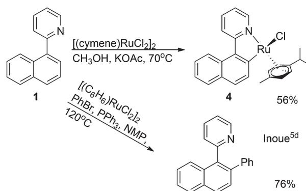
**Scheme 3** Isolation of metallacycle 4 – a possible intermediate in the catalytic arylation published by Inoue.<sup>5d</sup>
