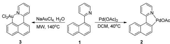
Scheme 2 Cyclometallation of 1 with Au and Pd precursors.
