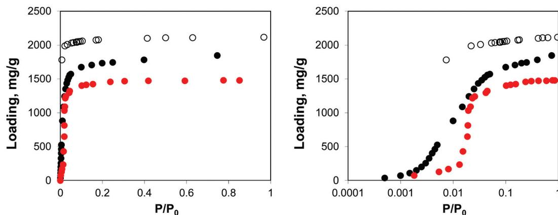
Fig. 3 Adsorption isotherms for argon at 78 K in IRMOF-1. Red symbols are the experimental results,<sup>7,26</sup> open symbols are unscaled simulation results from Dubbeldam and co-workers,<sup>26</sup> black symbols are from molecular simulations in this work. The panel on the right uses the logarithmic pressure scale.
