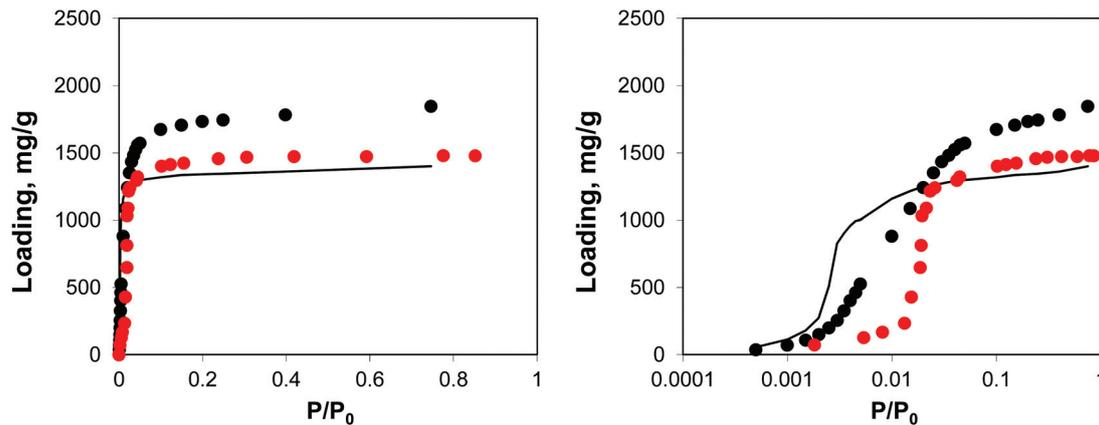
Fig. 12 Adsorption isotherms for argon at 78 K. Red symbols are the experimental results,<sup>7,26</sup> black symbols are from molecular simulations, black line corresponds to the system loaded with gold nanoclusters. The panel on the right uses the logarithmic pressure scale.
