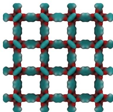
Fig. 2 Computer visualization of the ideal IRMOF-1 structure.  $2 \times 2 \times 2$  unit cells are shown under periodic boundary conditions. Cyan colour corresponds to the organic linkers, red colour indicates oxygen atoms associated with the zinc-containing vertices of the structure.
