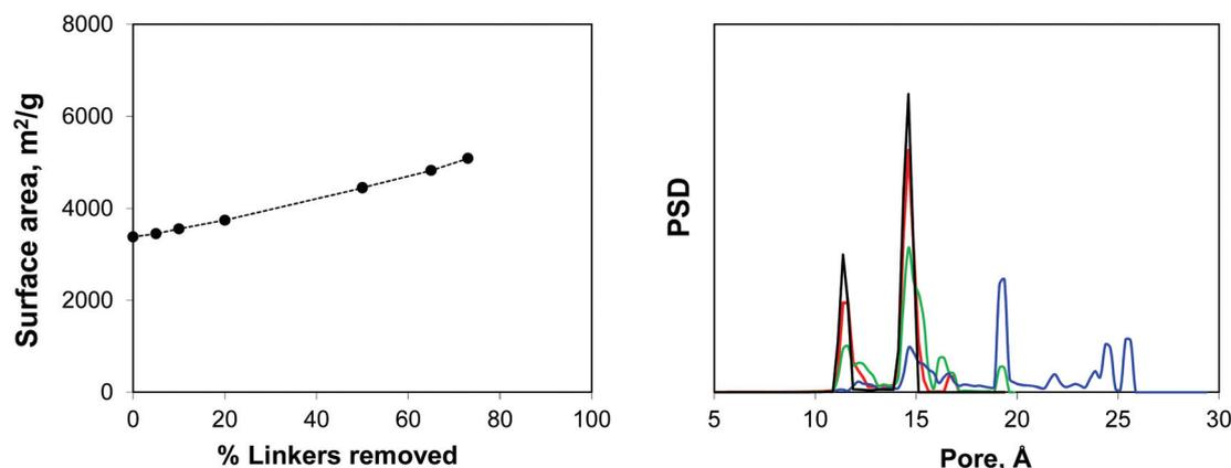
Fig. 4 On the left: accessible surface area ( $m^2 g^{-1}$ ) in IRMOF-1 as a function of the percentage of linkers removed. Line is for eye guidance only. On the right: geometric pore size distribution as a function of the percentage of linkers removed. Black line is for 0% (perfect crystal), red line is for 50%, green line is for 65% and blue line is for 73% linkers removed.
