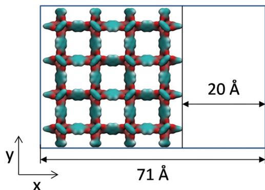
Fig. 7 Schematic depiction of a mesoporous model of IRMOF-1 considered here. In the  $x$  direction the system consists of alternating sheets of the IRMOF-1 crystal of two unit cells wide and gaps of 20 Å wide. The system is under periodic boundary conditions in the  $y$  and  $z$  directions.
