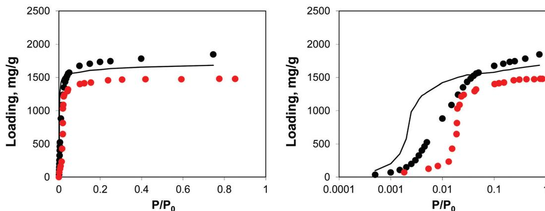
Fig. 10 Adsorption isotherms for argon at 78 K in IRMOF-1. Red symbols are the experimental results,<sup>7,26</sup> black symbols are from molecular simulations, black line corresponds to the system with residual DMF. The panel on the right uses the logarithmic pressure scale.
