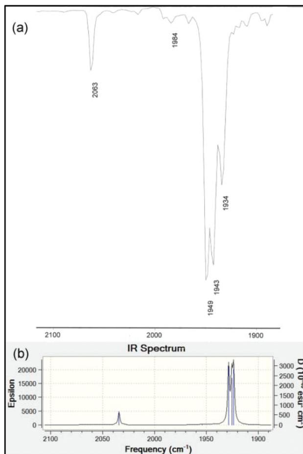
Fig. 6 (a) Experimental solution IR spectrum in the carbonyl stretching region of **10** measured dilute in hexane. (b) Computed gas-phase IR spectrum at the B3PW91/LANL2DZ level of theory (data in Table 3).
