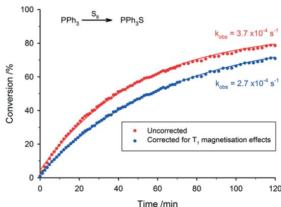
Fig. 6 Comparison between uncorrected and corrected reaction progress data of the oxidation of triphenylphosphine [ $T_1 = 15.6$  s] to triphenylphosphine sulphide [ $T_1 = 4.8$  s] from  $^{31}\text{P}$  FlowNMR accounting for incomplete pre-magnetisation (toluene, 25 °C, 30° pulse, inverse gated decoupling, 0.8 s acquisition time, 2 s relaxation delay). Both datasets corrected for relaxation delay quantification effects (see Experimental section for details).
