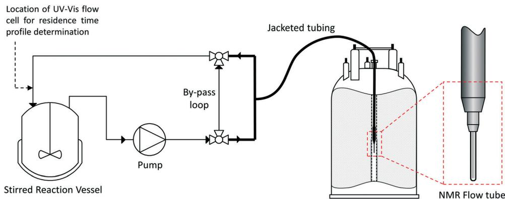
Fig. 1 Flow scheme and instrumentation diagram for the FlowNMR reaction monitoring apparatus (not to scale; for details see the Experimental section).
