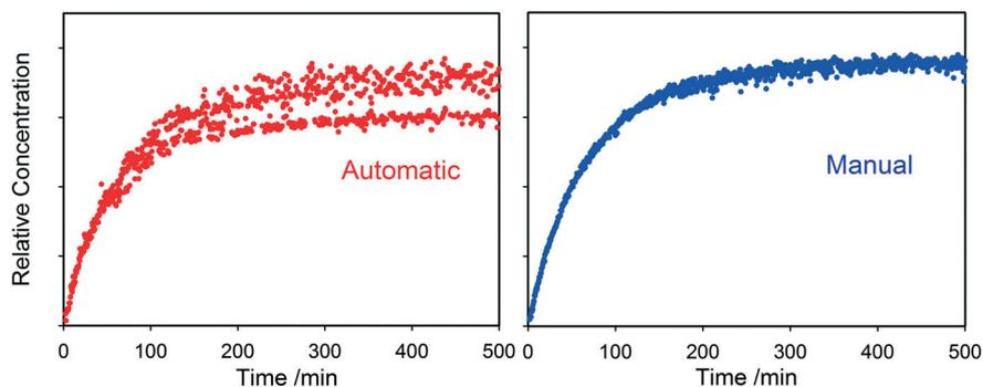
Fig. 12 Comparison between the same  $^1\text{H}$  reaction progress data processed using automatic phase and baseline corrections (left) and with manual refinement of parameters to reduce baseline distortions and data scatter (right). Note that a particularly noisy data set was chosen for illustration purposes, and higher quality reaction profiles are typically obtained from FlowNMR experiments (see e.g. Fig. 6 and 13).
