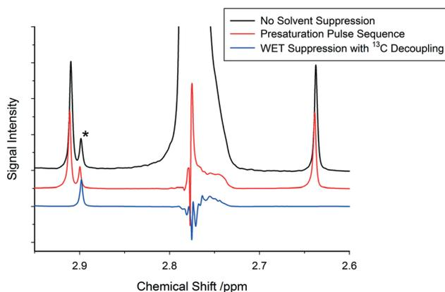
Fig. 11 Suppression of the acetonitrile  $\text{CH}_3$  peak in flow comparing a simple presaturation pulse sequence with a WET pulse sequence including  $^{13}\text{C}$  decoupling, leading to an approximately 500-fold reduction in peak intensity ( $500\text{ MHz}$ ,  $25^\circ\text{C}$ ,  $3.17\text{ s}$  acquisition time,  $4\text{ s}$  relaxation delay,  $4\text{ mL min}^{-1}$  flow rate). \*Solvent impurity peak not suppressed, demonstrating selectivity of WET suppression.
