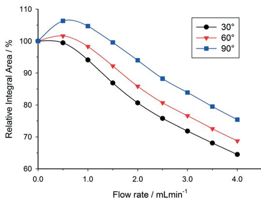
Fig. 10 Variation in  $^1\text{H}$  integral area of the acetone  $\text{CH}_3$  peak with increase in flow rate for different flip angles, showing increase in integral areas due to relaxation delay time effects for flip angles greater than  $30^\circ$  ( $25^\circ\text{C}$ ,  $3.2\text{ s}$  acquisition time,  $4\text{ s}$  relaxation delay).
