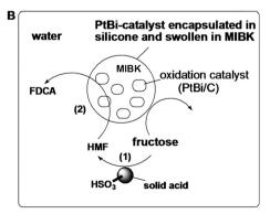
Fig. 7 (A) Membrane reactor: (step 1) HMF formation in the water phase, (step 2) diffusion of HMF in the MIBK phase, (step 3) HMF oxidation. (B) Batch reactor for direct transformation of fructose into FDCA: (step 1) acid-catalyzed dehydration of fructose to HMF, (step 2) diffusion of HMF into the silicone network and oxidation into FDCA. 121
