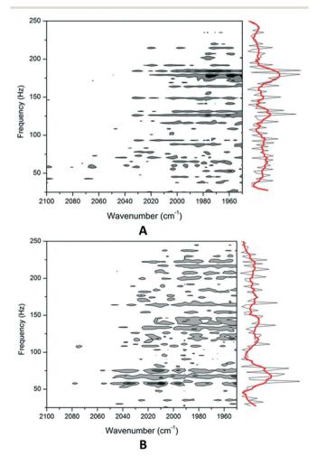
Fig. 2 2D PJAS-IR maps (at 300 °C) of CO adsorbed on Pt/ZSM-5: (A) Pt/Z-26-CIE and (B) Pt/Z-26-IWI.
