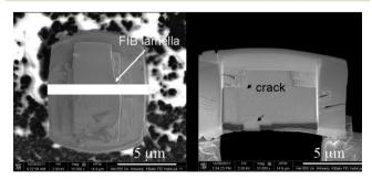
Fig. 3 SEM images of (left) the large coffin-shaped Z-1 ZSM-5 crystal and (right) the FIB lamella.
