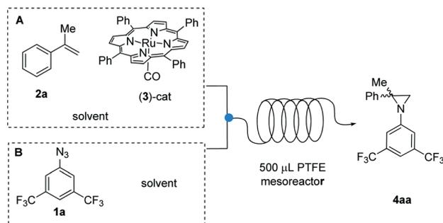
**Scheme 2** Reaction between azide **1a** and  $\alpha$ -methylstyrene **2a** promoted by  $[\text{Ru}(\text{TPP})(\text{CO})]$  catalyst **3** in a two-syringe continuous-flow system, using a 500  $\mu\text{L}$  PTFE mesoreactor.
