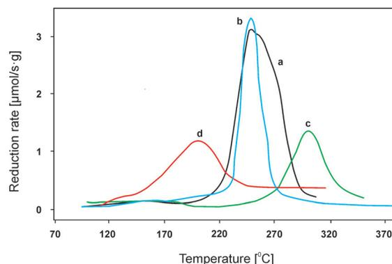
Fig. 2 Results of temperature-programmed reduction ( $\text{H}_2\text{-TPR}$ ) performed for  $\text{Mg-Cu-Al-O}_x$  ((a) 12.5 wt%, (b) 8.0 wt% and (c) 4.0 wt%  $\text{CuO}$ ) and  $\text{Cu/Mg-Al-O}_x$  ((d) 10.0 wt%) (adapted from ref. 41 with kind permission from Elsevier).
