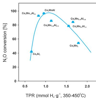
Fig. 8 Dependence of N<sub>2</sub>O conversion on the amount of reducible components in the interval of 350–450 °C. Reaction conditions: 0.1% N<sub>2</sub>O, He balance; total flow rate = 100 ml min<sup>-1</sup>; mass of catalyst = 100 mg; temperature = 450 °C (adapted from ref. 169 with kind permission from Elsevier).
