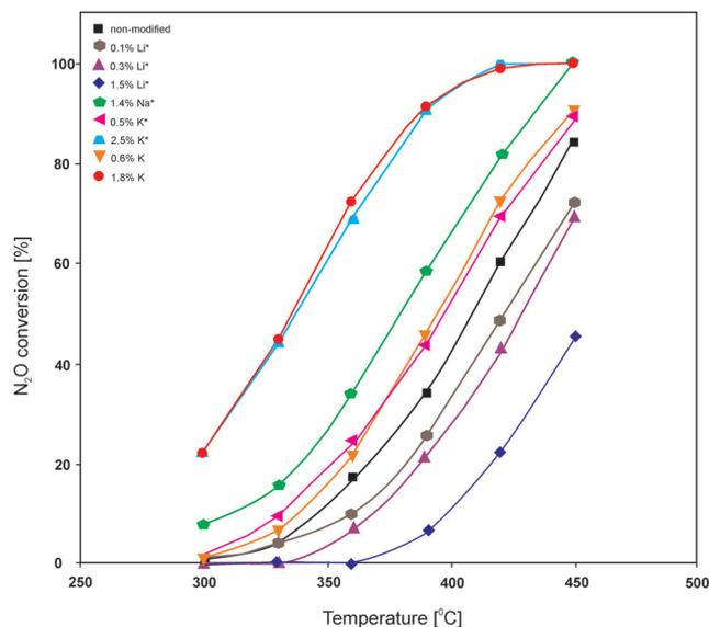
**Fig. 9** Results of catalytic tests performed for Co-Mn-Al-O<sub>x</sub> modified with Li, Na or K; alkali metals were added after coprecipitation of the precursors or by impregnation of calcined precursors (samples labelled as \*). Reaction conditions: 0.1% N<sub>2</sub>O, He balance; total flow rate = 100 ml min<sup>-1</sup>; mass of catalyst = 100 mg (adapted from ref. 163 with kind permission from Elsevier).
