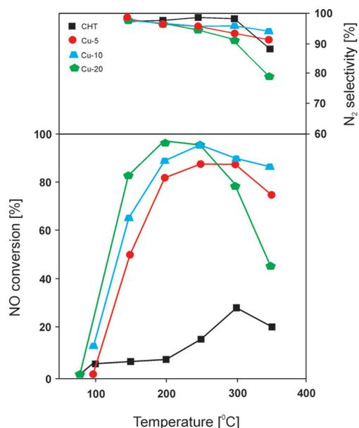
Fig. 3 Results of catalytic tests performed for Cu–Mg–Al–O<sub>x</sub>. Reaction conditions: 0.25% NO, 0.25% NH<sub>3</sub>, 2.5% O<sub>2</sub>, He balance; total flow rate = 40 ml min<sup>-1</sup>; mass of catalyst = 200 mg (adapted from ref. 66 with kind permission from Elsevier).
