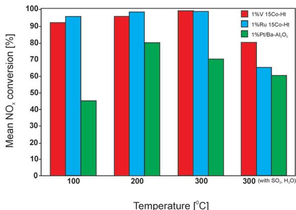
**Fig. 6** Results of catalytic tests performed for Mg–Co–Al–O<sub>x</sub>. Reaction conditions: lean (120 s): 13.0% O<sub>2</sub>, 0.053% NO, 0.005% C<sub>3</sub>H<sub>8</sub>; rich (60 s): 8.0% O<sub>2</sub>, 0.053% NO, 0.07% C<sub>3</sub>H<sub>8</sub>, N<sub>2</sub> balance; total flow rate = 650 ml min<sup>-1</sup>; mass of catalyst = 1000 mg (adapted from ref. 110 with kind permission from Elsevier).
