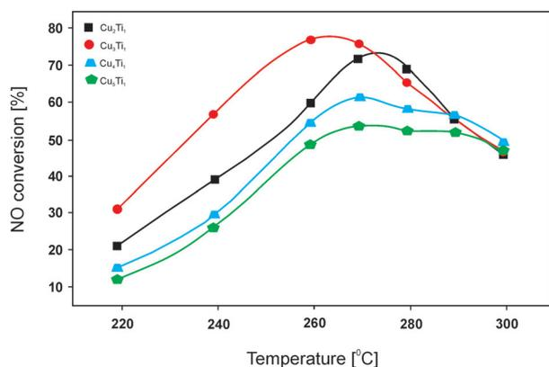
Fig. 5 Results of catalytic tests performed for Cu–Ti–O<sub>x</sub>. Reaction conditions: 0.1% NO, 0.1% C<sub>3</sub>H<sub>6</sub>, 1.0% O<sub>2</sub>, He balance; total flow rate = 100 ml min<sup>-1</sup>; mass of catalyst = 300 mg (adapted from ref. 83 with kind permission from Elsevier).
