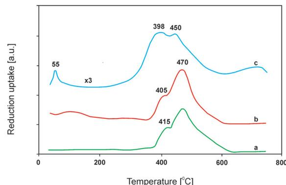
**Fig. 7** Results of temperature-programmed reduction (H<sub>2</sub>-TPR) performed for Mg–Fe–Al–O<sub>x</sub> (a), Mg–Zn–Al–Fe–O<sub>x</sub> (b) and Pd/K/Mg–Zn–Al–Fe–O<sub>x</sub> (c) (adapted from ref. 111 with kind permission from Elsevier).
