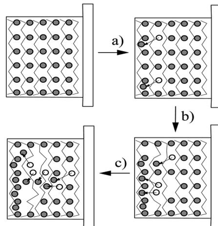
**Fig. 9** The different steps of the overoxidation process: (a) doping anion migration; (b) doping anion accumulation at the surface; (c) doping anion expulsion due to its hydrophobic character. The zig-zag lines stand by the PPy chains while grey circles represent the positions of the doping anions and the empty circles the previously occupied position and the arrows indicate the trajectory of the moved anion. (Reproduced with permission from ref. 10. Copyright 2005, Elsevier).
