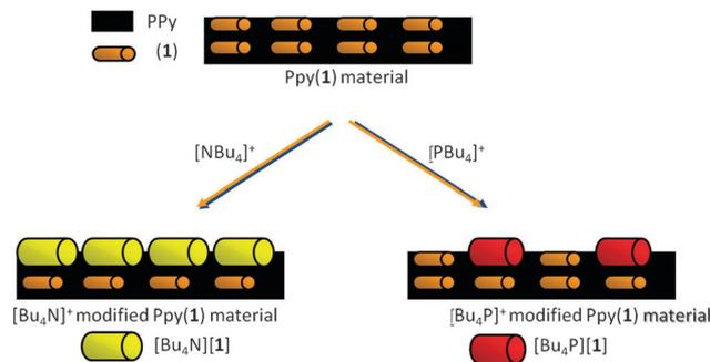
**Fig. 4** Graphical representation of the PPy(1) polymer modified by [NBu<sub>4</sub>]<sup>+</sup> and [PBu<sub>4</sub>]<sup>+</sup>.
