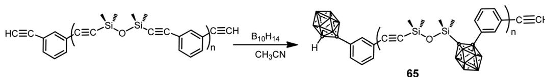
Scheme 20 Preparation of poly(siloxane-arylacetylene)s **65** from B<sub>10</sub>H<sub>14</sub>.
