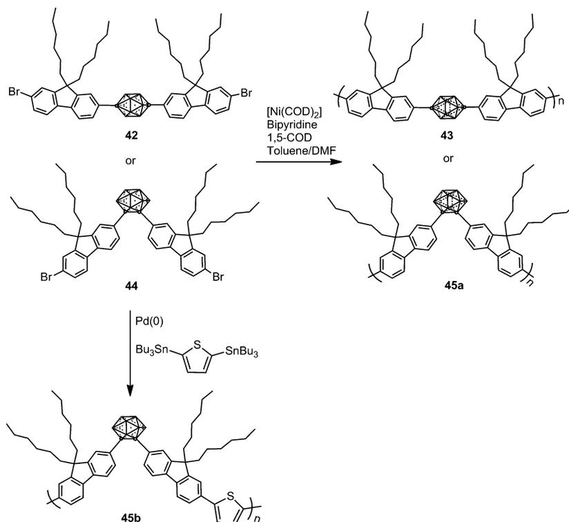
Scheme 8 Synthesis of polymers **43**, **45a** and **45b**.
