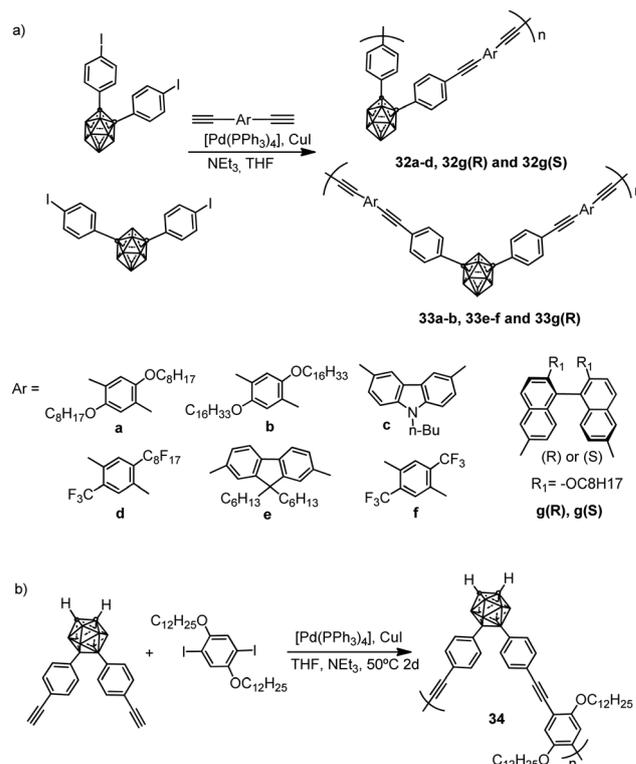
Scheme 3 (a) Polymers with *o*- and *m*-carborane linked by C<sub>c</sub>; (b) polymers with *o*-carboranyl linked by the B<sub>c</sub>.
