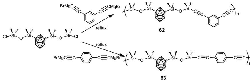
Scheme 18 Preparation of poly(carborane-siloxane arylacetylene) polymers **62** and **63**.
