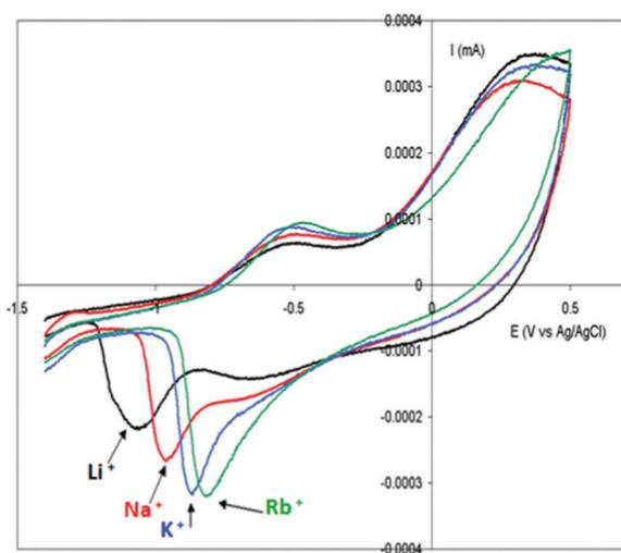
**Fig. 3** Cyclic voltammety of PPy(1) membranes in aqueous alkaline chlorides: LiCl 0.1 M; NaCl 0.1 M; KCl 0.1 M; RbCl 0.1 M; CsCl 0.1 M. Scan rate of electrode potential 20 mV s<sup>-1</sup>.
