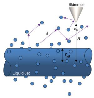
**Fig. 4** Evaporating molecules create a vapor cloud surrounding the liquid microjet. The number of vapor-vapor collisions over the distance R depends on both the mean free path  $\lambda$  and the jet radius  $r_{\rm iet}$ .
