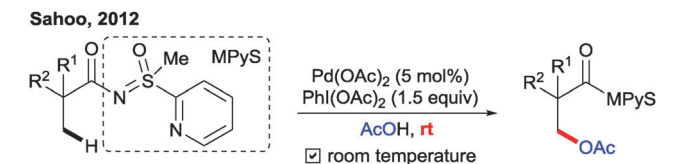
Scheme 32 A bidentate directing group as a handle for mild Pd-catalyzed aliphatic C–H activation. 80
