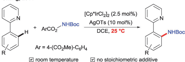
Scheme 56 Mild Ir-catalyzed amination with an electrophilic reagent. 123
