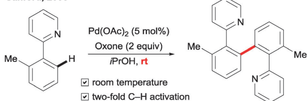
Scheme 9 Oxidative arene dimerization involving proposed C–H activation at Pd IV . 17
