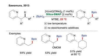
Scheme 17 Silica-supported Ir-based heterogeneous catalyst for the direct borylation of C(sp3)-H bonds.38
