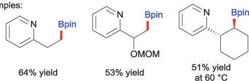
Scheme 17 Silica-supported Ir-based heterogeneous catalyst for the direct borylation of C(sp 3 )–H bonds. 38
