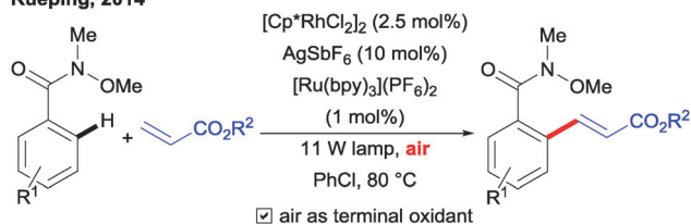
Scheme 76 Rh III -catalyzed oxidative olefination using photoredox catalysis to replace stoichiometric amounts of oxidant with air. 156
