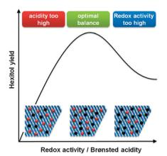
Fig. 7 Influence of the balance between redox (black sites) and Brønsted (red) sites on the hexitol selectivity during hydrolytic hydrogenation of cellulose
