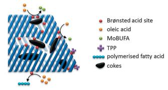
Fig. 5 Schematic presentation of the pore mouth catalytic conversion of oleic acid over Brønsted acidic zeolites towards MoBUFA in the presence
