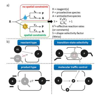
(a) The most basic definition of shape-selectivity, defined when S > 1. The drop represents reaction in absence of structural constraints on molecular motion or formation. (b) The 3 foremost types of shape-selectivity along with molecular traffic control.
