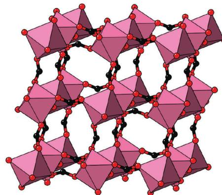
Fig. 8 Representation of the crystal structure of  $[\text{NMe}_2\text{H}_2]\text{Mn}[\text{HCOO}]_3$ , as reported in ref. 25. Mn coordination polyhedra are shown in pink, O atoms as red spheres, and C atoms as black spheres.  $[\text{NMe}_2\text{H}_2]^+$  cations and H atoms have been omitted for clarity. Here the shift distortions are associated with macroscopic shear of the lattice.
