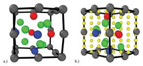
Fig. 1 (a) Structure matched  $\rm Y_2Ti_2O_7$  oxide nanocluster embedded in Fe and (b) 8  $\times$  8 mesh used for the calculation of the potential energy landscape in the (1 –1 0) plane. Red, blue, green, silver, and yellow atoms represent Y, Ti, O, Fe, and He respectively (the iron matrix is not fully shown for clarity).
