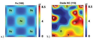
Fig. 7 Potential energy landscape in the (a) (1 0 0) plane of BCC Fe and (b) (1 -1 0) plane of the oxide NC embedded in BCC Fe. Approximate locations of atomic species in the immediate vicinity of potential energy maxima are labeled. Both potential energy landscapes have been calculated in the same supercell, and both plot have the same energy reference.
