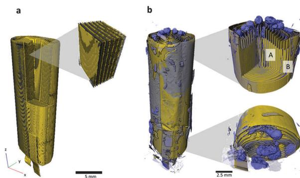
Fig. 3 (a) 3D reconstruction of the pouch cell in its fresh state. The LiCoO<sub>2</sub> electrode is displayed as grey, and the copper current collector and tabs are shown in yellow. (b) 3D reconstruction showing the pouch cell after overcharge-induced thermal runaway. Copper and LiCoO<sub>2</sub> phases are labelled as yellow and aluminium is shown in blue. Samples were taken from regions A and B for further analysis using micro-X-ray CT.
