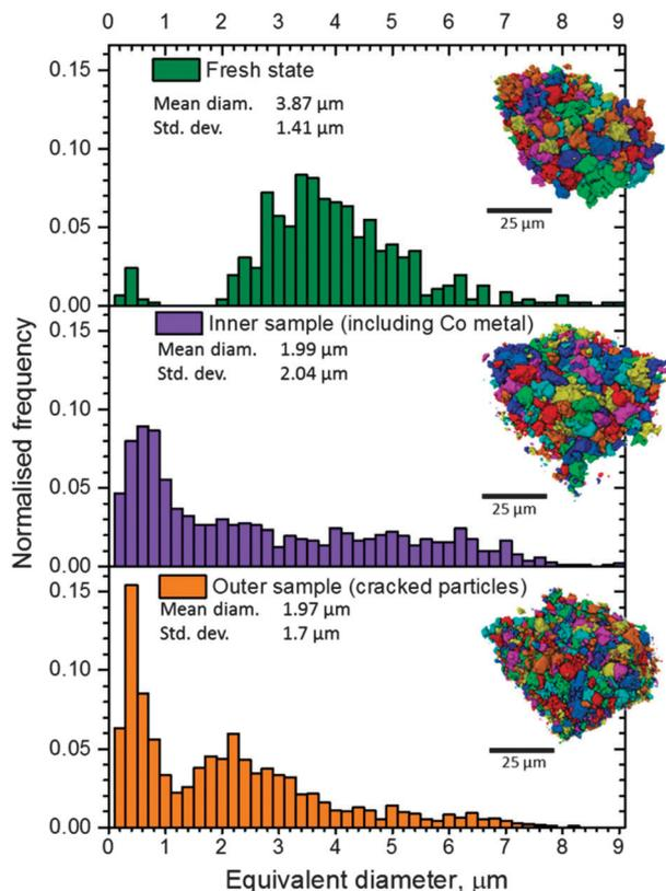
Fig. 8 Particle size distributions for  $\text{LiCoO}_2$  particles from a fresh sample (top), a sample taken from the inner regions of the failed overcharged cell showing evidence of complete reduction to Co metal (middle), and a sample taken from the outer region of the failed overcharged cell showing evidence of particle cracking with no formation of Co (bottom).
