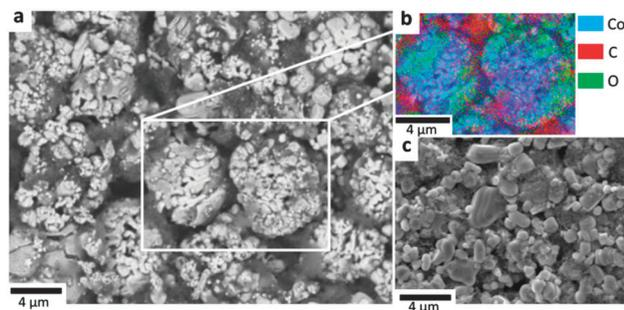
Fig. 6 (a) SEM micrograph of the  $\text{LiCoO}_2$  material after overcharge and thermal runaway, (b) EDS of the highlighted region showing that the surface layer consists of Co metal, and (c) SEM micrograph of the fresh  $\text{LiCoO}_2$  particles.
