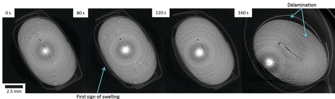
Fig. 2 Time-stamped horizontal slices taken from sequential tomograms during electrical overcharge of the LiCoO<sub>2</sub> cell. Pouch swelling begins after 80 s (blue arrow), and the electrode layers begin to deform and delaminate after 160 s. The LiCoO<sub>2</sub> electrode also delaminates from the Al current collector after 160 s (blue arrow pointing to inner region).
