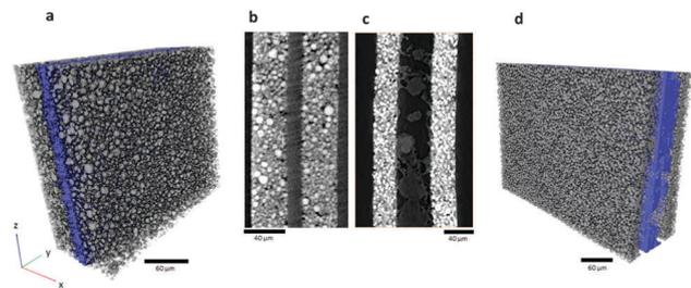
Fig. 4 (a) 3D reconstruction of aluminium current collector (blue) coated with LiCoO<sub>2</sub> (grey) in its fresh state alongside an XZ orthoslice (b). (c) and (d) show an XZ orthoslice and 3D reconstruction of the current collector and the remains of LiCoO<sub>2</sub> after thermal runaway.
