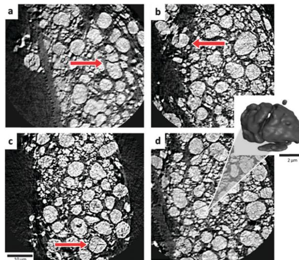
Fig. 7 (a–d) Orthoslices highlighting cracked  $\text{LiCoO}_2$  particles. Sample was extracted from the outer region labelled as B in Fig. 3. Inset: An isolated 3D volume of the cracked particle in (d).
