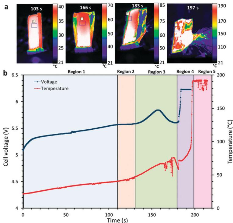
**Fig. 1** (a) Sequence of time-stamped thermal images showing the increasing surface temperature of the LiCoO<sub>2</sub> pouch cell leading up to thermal runaway. The average temperature within the labelled square is plotted. (b) Plot of the cell voltage and surface temperature, leading up to and during thermal runaway. The battery was charged at a constant current of 3 A (18.75 C), from 100% SOC (4.2 V) until failure. Real time thermal images are presented in Movie S1 (ESI†).
