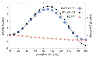
Fig. 5 Potential energy surface (PES) obtained using the modified force field (black squares), DFT calculations (blue circles), the PCFF\* force field (red triangles). The modified force field gives reasonable agreement with the B3LYP+D3. Dispersion interaction between the methyl side chains leads to cis conformation (180°) preference over trans conformation (0°).
