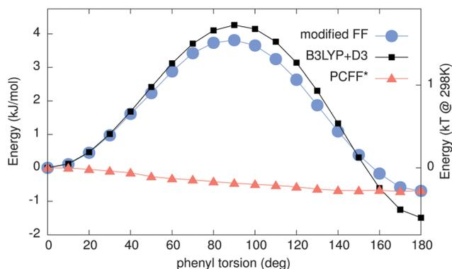
Fig. 5 Potential energy surface (PES) obtained using the modified force field (black squares), DFT calculations (blue circles), the PCFF\* force field (red triangles). The modified force field gives reasonable agreement with the B3LYP+D3. Dispersion interaction between the methyl side chains leads to *cis* conformation ( $180^\circ$ ) preference over *trans* conformation ( $0^\circ$ ).
