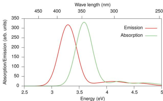
Fig. 9 Optical absorption (blue) and emission (blue) spectra of 2,5-dinonyl-10-PPE in toluene as obtained from GW-BSE/MM calculations using fragment based re-mapping. Both spectra are averages over 11 snapshots taken every 1 ps, respectively. A Stokes shift (red shift) of 0.29 eV is found, which compares well to experimental observations of 0.3–0.4 eV.<sup>48</sup>
