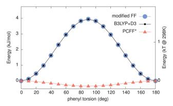
Fig. 3 Potential energy surface (PES) obtained by MM/MD and quantum mechanical (QM) calculations. Red triangles show the PES calculated using the PCCF\*<sup>56,57</sup> force field. Black squares are the QM results using B3LYP+D3. Blue circles show the PES obtained using our new modified force field. The modified force field and B3LYP+D3 are in excellent agreement.
