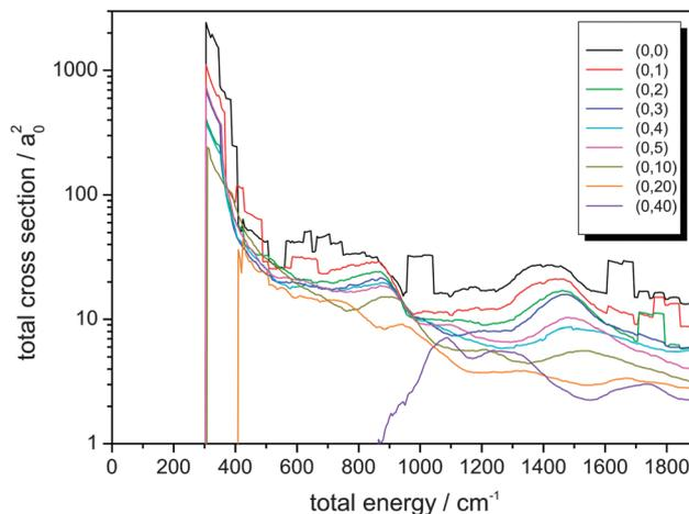
**Fig. 1** Integral reaction cross sections summed over all product states for the reaction Cl<sup>-</sup> + CH<sub>3</sub>Br ( $v,j$ ) → ClCH<sub>3</sub> + Br<sup>-</sup>, for different initial rovibrational states ( $v = 0, j$ ) with initial rotational excitation of CH<sub>3</sub>Br up to  $j = 40$ .
