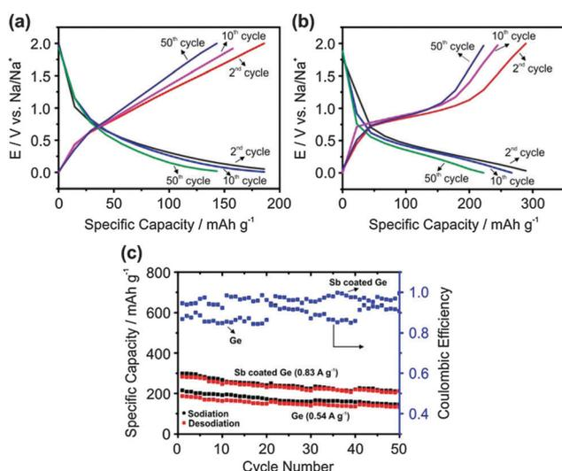
Fig. 3 Charge discharge curves for 2nd, 10th and 50th cycles for (a) electrodeposited Ge at 0.54 A g<sup>-1</sup>; (b) Sb modified Ge at 0.83 A g<sup>-1</sup>; (c) 50 charge–discharge cycles of electrodeposited Ge and Sb modified Ge. The first charge–discharge cycle was run at 0.02C to form a stable SEI layer.
