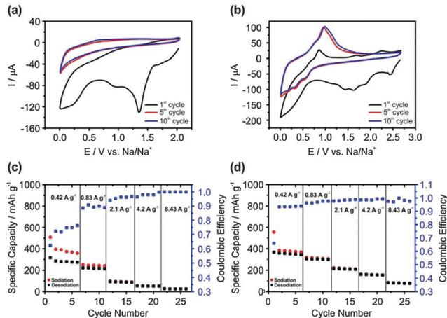
**Fig. 2** (a) CV of electrodeposited Ge in 1 M NaFSI-[Py<sub>1,4</sub>]FSI at a scan rate of 1  $\text{mV s}^{-1}$ ; (b) CV of Sb modified Ge by electrodeless deposition, in 1 M NaFSI-[Py<sub>1,4</sub>]FSI at a scan rate of 1  $\text{mV s}^{-1}$ ; (c and d) charge–discharge cycles at various current densities on electrodeposited Ge and Sb modified Ge, respectively. The first charge–discharge cycle was run at 0.02C to form a stable SEI layer.
