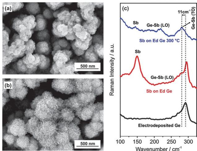
**Fig. 1** (a) Microstructure of electrodeposited Ge; (b) SEM of electrodeless deposited Sb on Ge from 0.1 M  $\text{SbCl}_3$ -[Py<sub>1,4</sub>]TFSI; (c) Raman spectra of electrodeposited Ge (black line), electrodeless deposited Sb on Ge (red line) and after annealing to 300 °C (blue line).
