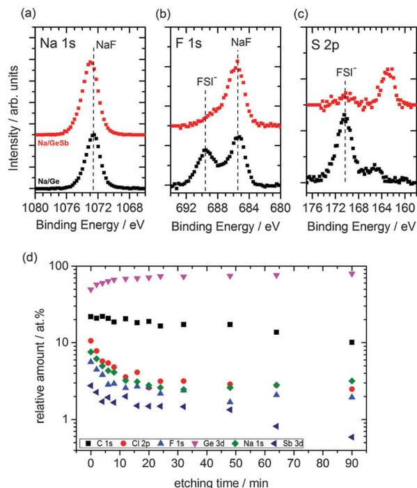
Fig. 4 (a–c) XPS detailed spectra (Na 1s, F 1s and S 2p) of electrodeposited Ge (black) and Sb modified Ge (red) after 50 charge–discharge cycles in 1 M NaFSI-[Py<sub>1,4</sub>]FSI; (d) stoichiometry of surface components from XPS survey spectra after sputter etching with 2 keV Ar<sup>+</sup> ions for Sb modified Ge sample after cycling.
