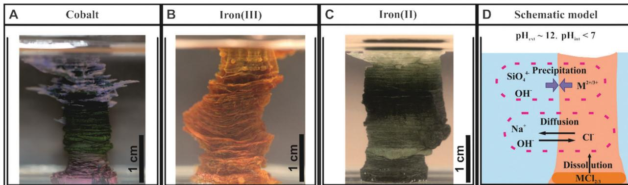
Fig. 1 Photographs of single macroscopic silica garden tubes obtained by controlled addition of sodium silicate solution to pressed pellets of (A)  $\text{CoCl}_2$ , (B)  $\text{FeCl}_3$  and (C)  $\text{FeCl}_2$ . (D) Scheme illustrating the situation at the end of the growth process, where the formed membrane encloses an inner acidic solution rich in metal cations that is surrounded by an outer alkaline solution containing mainly sodium and silicate ions.
