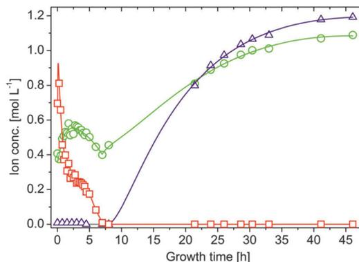
Fig. 3 Long-term evolution of iron (squares), sodium (circles) and silicate (triangles) ion concentrations in the interior solution of  $\text{FeCl}_3$ -based silica gardens. Note that the full lines are only meant to serve as a guide to the eye and do not rely on a distinct physical model.
