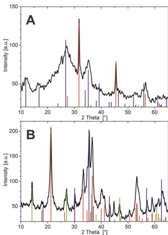
**Fig. 5** XRD patterns of silica garden tubes prepared with pellets of (A) FeCl<sub>3</sub> and (B) FeCl<sub>2</sub>. Vertical lines mark signals belonging to the different occurring crystalline phases according to (A) blue: FeOOH (akaganeite-M; JCPDS No. 34-1266), red: NaCl (JCPDS No. 5-628), and (B) red: FeOOH (goethite; JCPDS No. 29-713), green: FeOOH (lepidocrocite; JCPDS No. 8-98), and blue: Fe<sub>3</sub>O<sub>4</sub> (magnetite; JCPDS No. 19-629).
