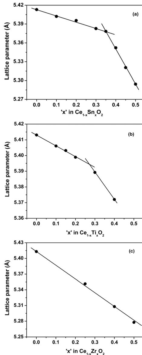
Fig. 2 Lattice parameter vs. substituent concentration in (a)  $\text{Ce}_{1-x}\text{Sn}_x\text{O}_2$ , (b)  $\text{Ce}_{1-x}\text{Ti}_x\text{O}_2$  and (c)  $\text{Ce}_{1-x}\text{Zr}_x\text{O}_2$  solid solutions.
