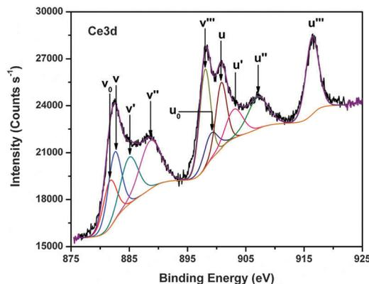
Fig. 5 Curve-fitted Ce3d core level spectrum of  $\text{Ce}_{0.65}\text{Sn}_{0.35}\text{O}_{2-\delta}$ .
