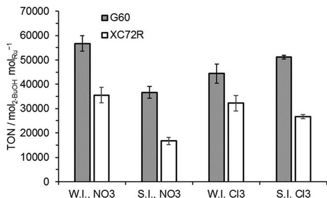
Fig. 4 The effect of different carbons, precursors, and preparation methods on Ru/C catalysts for 2-butanone hydrogenation. WI = wet impregnation; SI = sol immobilisation; NO<sub>3</sub> = Ru(NO)(NO<sub>3</sub>)<sub>3</sub> precursor; Cl<sub>3</sub> = RuCl<sub>3</sub> precursor. Reaction conditions: 110 °C, 1 bar H<sub>2</sub>, 0.5 h, 5 wt% 2-butanone in H<sub>2</sub>O, 0.05 g of catalyst.
