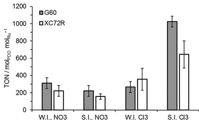
Fig. 3 The effect of different carbons, precursors, and preparation methods on Ru/C catalysts for lactic acid hydrogenation. WI = wet impregnation; SI = sol immobilisation; NO<sub>3</sub> = Ru(NO)(NO<sub>3</sub>)<sub>3</sub> precursor; Cl<sub>3</sub> = RuCl<sub>3</sub> precursor. Reaction conditions: 125 °C, 35 bar H<sub>2</sub>, 2.5 h, 5 wt% lactic acid in H<sub>2</sub>O, 0.1 g of catalyst.
