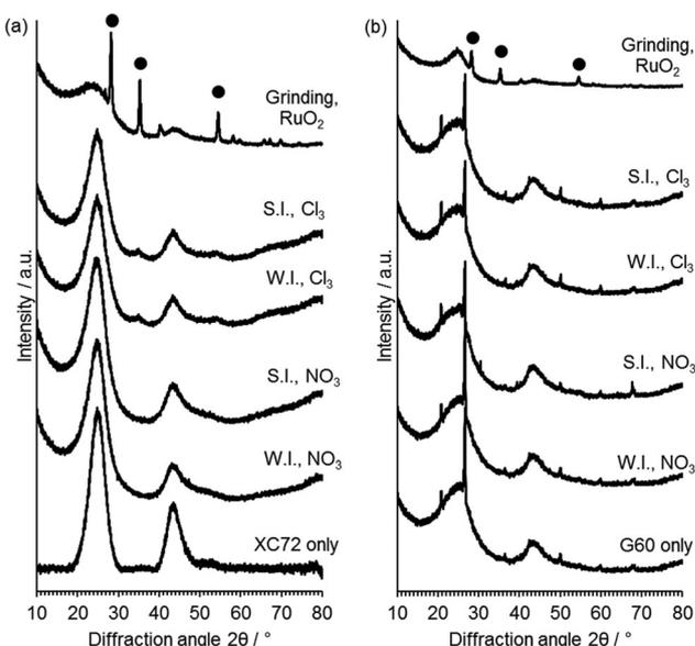
Fig. 5 XRD patterns for 1 wt% Ru/C catalysts prepared using (a) XC72 carbon and (b) G60 carbon. ● RuO<sub>2</sub>. WI = wet impregnation; SI = sol immobilisation; NO<sub>3</sub> = Ru(NO)(NO<sub>3</sub>)<sub>3</sub> precursor; Cl<sub>3</sub> = RuCl<sub>3</sub> precursor.
