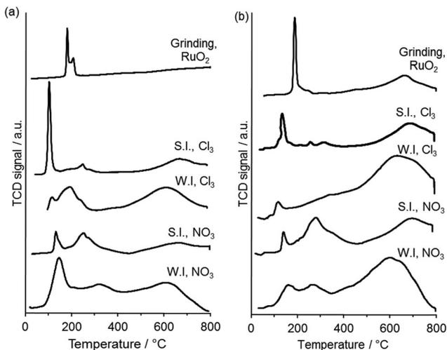
Fig. 6 TPR profiles for 1 wt% Ru/C catalysts prepared using (a) XC72R carbon and (b) G60 carbon. WI = wet impregnation; SI = sol immobilisation; NO<sub>3</sub> = Ru(NO)(NO<sub>3</sub>)<sub>3</sub> precursor; Cl<sub>3</sub> = RuCl<sub>3</sub> precursor.
