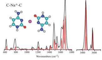
Fig. 4 Experimental IRMPD spectra of C-Li<sup>+</sup>-C and C-Na<sup>+</sup>-C in the  $600-1800~\text{cm}^{-1}$  and hydrogen stretching regions (black trace), compared with the computed spectra for the  $C1_{N3O}C1_{N3O}$  isomers (red trace) of these complexes.
