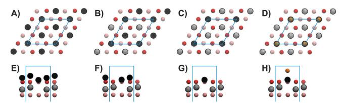
Fig. 1 Structural models of the TM structure (A + E), the DM structure (B + F), the SM structure (C + G) and the V $\equiv$ O terminated structure (D + H). Images (A) through (D) show top views of the respective surfaces while images (E) through (H) show sideviews visualizing the stacking sequence. Color-coding: surface V - black, bulk V - grey, surface O - red, bulk O - pink, vanadyl O - orange; unit cells indicated in blue.
