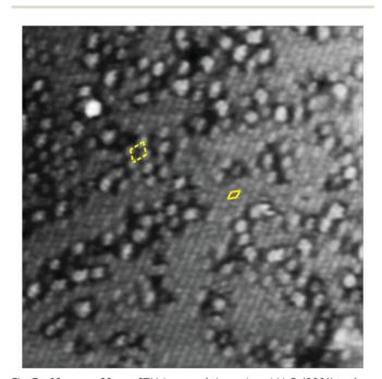
Fig. 3 20 nm  $\times$  20 nm STM image of the reduced  $V_2O_3(0001)$  surface (145 mC c.e.d.), +1 V, +0.1 nA. The apparent unit meshes are indicated by rhombi drawn with full (flat surface) and broken (rough surface) lines. The image has been FFT-filtered. See the ESI† for the raw image and Fourier transforms
