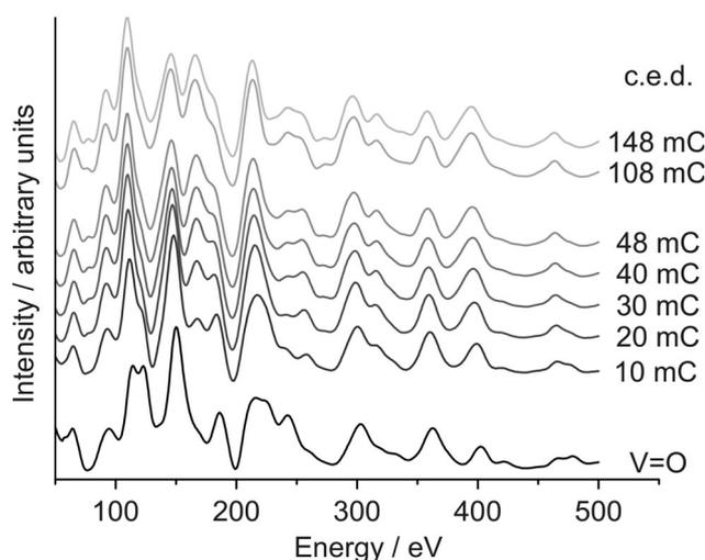
Fig. 2  $I/V$ -LEED curves showing the stepwise reduction of the  $V_2O_3(0001)$  surface. The cumulative electron dose is indicated next to the curves.
