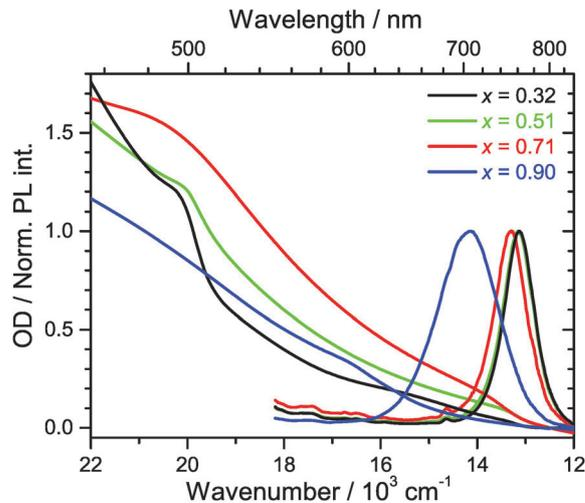
Fig. 2 Steady-state absorption (left) and photoluminescence spectra (right) of  $(\text{MAI})_x(\text{PbI}_2)_{1-x}/\text{TiO}_2/\text{glass}$  prepared using different initial mole fractions  $x$  of MAI. Black: 0.32, green: 0.51, red: 0.71, blue: 0.90. For the sake of an easier comparison, absorption spectra are set to zero at 840 nm. Photoluminescence spectra are normalized to their peak amplitude.
