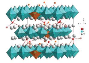
Fig. 2 Random step of the MD calculation on the  $(2\sqrt{2}, 2\sqrt{2}, 1)$  supercell of  $Nd_2NiO_{4.25}$  at T=310 K.  $NiO_6$  polyhedra are depicted in blue, while square-pyramid  $NiO_5$  polyhedra are in orange. Excess oxygen atom in an interstitial site is in red and bound to its four apical oxygen neighbours. Apical-interstitial oxygen pair in saddle state is in orange and bound to its first neighbour nickel atom.
