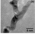
Fig. 2 Ag nanowires synthesized in He<sub>N</sub> ( $\bar{N} \approx 1.7 \times 10^{10}$ ), deposited and imaged on a LN<sub>2</sub> cooled (a-c) TEM grid. Continuous branched wires (a) show polycrystalline domains in HRTEM mode (b)
