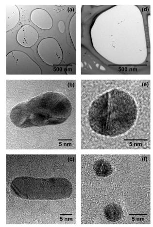
Fig. 3 Chains of Ag segments resulting from the breakup of nanowires as depicted in Fig. 2. Left column: (a) heavy doping of the droplet ( $\alpha = 0.75$ ). HRTEM measurements reveal either polycrystalline morphology (b) or large monocrystalline domains (c). Right column: (d) weak doping ( $\alpha = 0.2$ ). Silver segments resulting from the breakup of small nanowires often exhibit fivefold symmetry, i.e. icosahedral ((e), top of (f)) or decahedral (bottom of (f)) morphologies.
