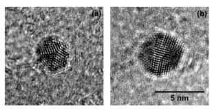
Fig. 1 Decahedral (a) and icosahedral (b)  $Au_n$  synthesized in  $He_N$  free from vortices ( $\overline{N} \approx 7 \times 10^6$  atoms), observed after deposition on a TEM substrate. The morphologies found agree well with those of Ag<sub>n</sub> produced under comparable conditions.<sup>30</sup> Scale is the same for both images.
