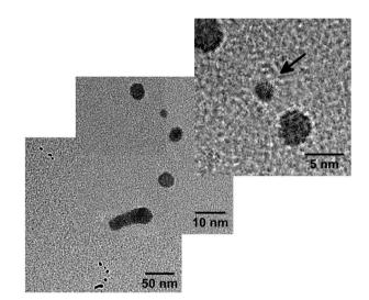
Fig. 5 Segmented Au nanowire resulting from very weak doping ( $\alpha$  = 0.04). The arrow marks a small decahedral cluster in the HRTEM image.
