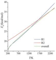
Fig. 3 Activation energies (kcal mol<sup>-1</sup>) for forward reactions (R1) and (R2) and the overall reaction at various temperatures.
