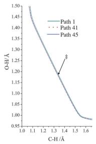
Fig. 9 Minimum energy path for paths 1, 41, and 45, where we show the breaking C-H bond distance and the forming H-O bond distance. Note that all three paths are shown, but as far the forming and breaking bond distances are concerned, the paths are so similar as to be hard to distinguish on the plot. The locations of the transition structures along the paths are similar for the three paths and are indicated by ‡.
