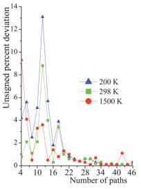
Fig. 12 Unsigned percent deviations of the generalized transmission coefficients for reaction (R1). The number of paths included (P) is the abscissa. The paths are indexed 1–46, with path numbering in order of increasing classical barrier height. The top figure is the deviation between including P paths and including all N paths. The bottom figure is the deviation between including P paths and including P paths. See eqn (13) and (14).
