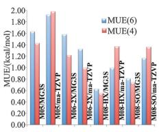
Fig. 1 Mean unsigned errors (MUEs) in kcal mol<sup>-1</sup> computed based on M08-HX/MG3S geometries using various methods, with respect to CCSD(T)-F12a/iun-cc-pVTZ as benchmark.
