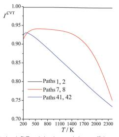
Fig. 4 Calculated CVT variational transmission coefficients at various temperatures (K) for different paths for reaction (R1): (CH<sub>3</sub>)<sub>3</sub>COH + HO<sub>2</sub> $^{\bullet}$   $\rightarrow$  CH<sub>2</sub> $^{\bullet}$ (CH<sub>3</sub>)<sub>2</sub>COH + H<sub>2</sub>O<sub>2</sub>.
