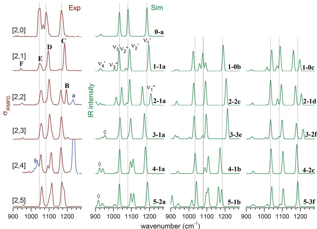
Fig. 6 Experimental IRMPD (left) and simulated B3LYP/def2-TZVP harmonic vibrational spectra (right) in the sulfate stretching region of  $(\text{NaSO}_4^-)_2(\text{H}_2\text{O})_n$  complexes with  $n = 0-5$  (denoted as  $[2,n]$ ). The corresponding structures are illustrated in Fig. 5. Contributions of the monomer species to the IRMPD spectra are highlighted (blue trace) and labelled with small letters.
