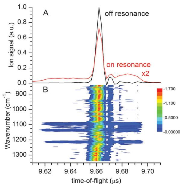
Fig. 2 TOF mass spectra measured after irradiation in the sulfate stretching region showing the effect of ion repulsion in-between the [1,0] photofragment ions upon photodissociation of [2,0] parent ions. Note, parent and fragment ions have identical *m/z* ratios. (A) Wavenumber-integrated TOF mass spectra measured off (black) and on (red) resonance. (B) 2D plot of the ion signal vs. FELIX wavenumber and ion TOF.
