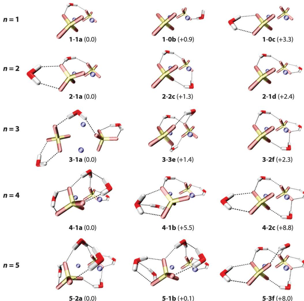
Fig. 5 B3LYP/def2-TZVP minimum-energy structures of the  $(\text{NaSO}_4^-)_2(\text{H}_2\text{O})_n$  complexes with  $n = 1-5$ . Relative energies (with ZPE correction) are given in  $\text{kJ mol}^{-1}$ .
