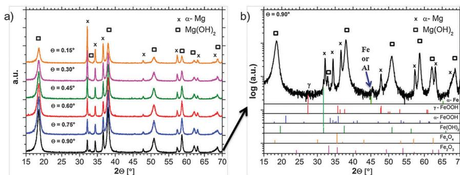
Fig. 8 (a) GIXRD pattern (measured *in situ*) after the formation of the dark area on Mg-65 ppm Fe in 0.5% NaCl solution showing the growth of  $\text{Mg}(\text{OH})_2$ . (b) GIXRD diffraction patterns measured at an incident angle of  $0.90^\circ$  (logarithmic scale) including the indication of probable phases.
