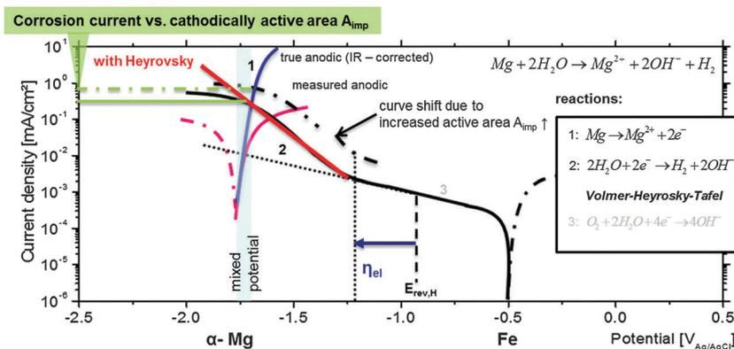
Fig. 9 Applied mixed potential theory, corrosion current density as a result of occurring reactions, the overpotential  $\eta_{el}$  vs.  $E_{rev,H}$ , the amount of cathodically active area  $A_{imp}$ , and its relation to single polarization curves. The RHE potential is indicated as well.
