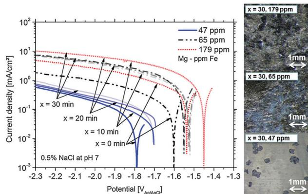
Fig. 1 Enhanced cathodic activity after anodic potentiostatic polarization for  $x = 0, 10, 20, 30$  minutes at  $+100$  mV vs. OCP for pure Mg containing different Fe levels and their surface appearance after  $x = 30$  min (initially all had a shiny surface).
