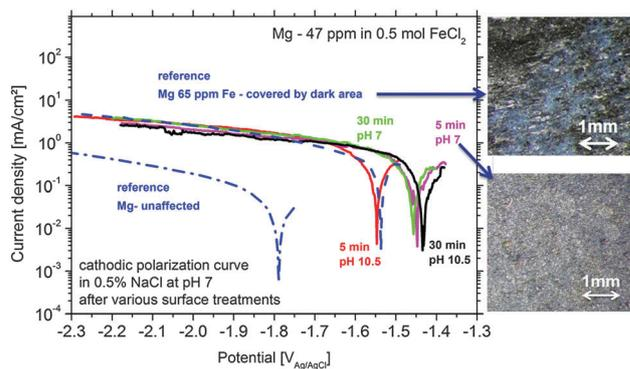
Fig. 3 Increased cathodic activity of Mg-47 ppm Fe samples after immersion treatments in 0.5 M  $\text{FeCl}_2$  solution for 5 and 30 min at pH 7 and 10.5. For comparison the initial bare- and corroded Mg-65 ppm Fe with the fully corroded surface are shown. The dark surface appearance of two test samples is shown by optical micrographs (initially all had a shiny surface).
