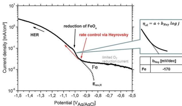
Fig. 10 Cathodic polarization curve on Fe in 90% deaerated alkaline 0.5 wt% NaCl solution (pH = 10.5) simulating the conditions during Mg corrosion. The pseudo-Tafel slope  $b_{Hey}$  in the Heyrovsky range follows the relation  $2 \times 2.303RT/F \leq b_{Hey} \leq 3 \times 2.303RT/F$ .<sup>83</sup>  $E_{rev,H}$  and the (virtual) hydrogen reduction related curve are adapted from the study of Chialvo *et al.*<sup>78</sup> Contribution to the current due to iron oxide reduction is labeled.
