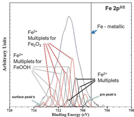
Fig. 4 Fe 2p<sub>3/2</sub> XPS spectra (Shirley background corrected) of the Mg-47 ppm Fe sample after immersion in 0.5 molar FeCl<sub>2</sub> solution for 5 min at initial pH 7 validated deposition of the Fe rich phase. Multiplet fitting according to the study of Grosvenor *et al.*<sup>57</sup> is implemented as well. Differentiation between  $\alpha$  and  $\gamma$  modifications of Fe<sub>2</sub>O<sub>3</sub> and FeOOH, respectively, is not indicated.
