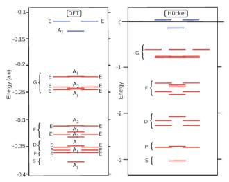
Fig. 3 Diagrams of the energetic levels for the  $C_{50}$  isomer  $D_3$ : on the left, the orbital scheme obtained from the DFT B3LYP/6-31G\* optimization and from Hückel theory on the right. The occupied orbitals are red, the unoccupied blue. Molecular orbital symmetry labels are also shown. The shells are indicated with brackets.
