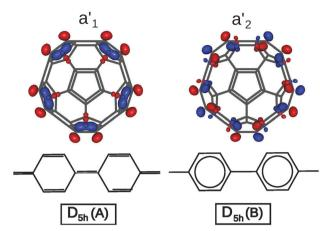
Fig. 2 Bond alternation in the equatorial belts for the A (Fries) and B (Clar) isomers of  $C_{50}$ , and orbital pictures of the frontier molecular orbitals (A isomer: a<sub>1</sub>' HOMO, a<sub>2</sub>' LUMO).
