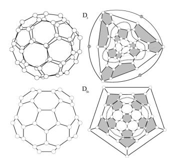
Fig. 1  $C_{50}$  isomers  $D_3$  and  $D_{5h}$  viewed from the main symmetry axes and their Schlegel projections. Dashed lines mark the equatorial regions of each molecule. Pentagons are colored in grey, and on the  $D_3$  figure, atom 5 is shaded.
