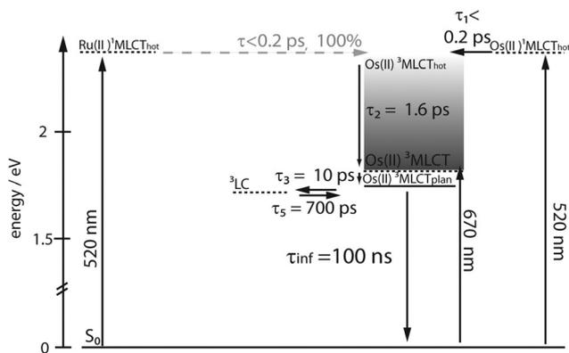
**Scheme 2** Proposed relaxation scheme for **RuOs**, solid lines define energy levels with defined energetic positions, while dashed lines define excited states, the energy of which can only be indirectly inferred or depends on the excitation wavelength, processes in grey are not directly observable in the data.
