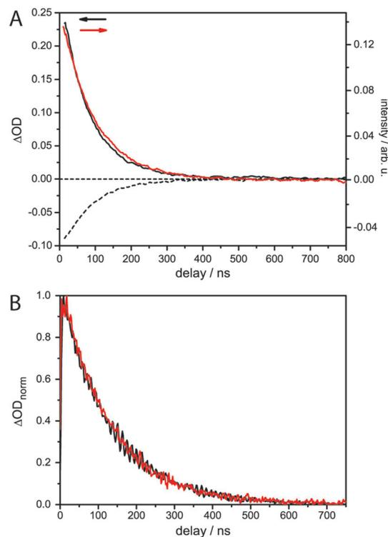
**Fig. 3** (A) Transient absorption kinetics of **RuOs** at selected probe wavelengths: 450 nm (dash/black), 590 nm (solid/black) and emission decay at 750 nm (red solid). (B) Direct comparison of the decay kinetics at 600 nm probe wavelength for **Ru** (black) and **RuFeRu** (red).
