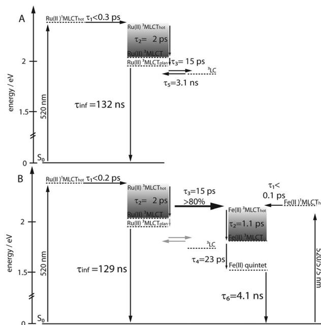
**Scheme 1** Proposed relaxation schemes for **Ru** and **RuFeRu**, solid lines define energy levels with defined energetic positions, while dashed lines define excited states, the energy of which can only be indirectly inferred or depends on the excitation wavelength, processes in grey are not directly observable in the data.
