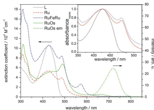
Fig. 2 Steady-state absorption spectra of **Ru**, **RuFeRu** and **RuOs** and emission spectrum of **RuOs** after excitation at 488 nm in aerated acetonitrile. For comparison the absorption spectrum of the bridging ligand **L** in dichloromethane is given. The inset shows the normalized absorption spectra of **L**, **Ru** and **RuFeRu** for comparison of the position of the LC absorption band.
