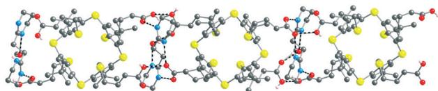
Fig. 7 Solid state structures of the 1D H-bonded  $[5^{2-}\text{-}A^{2+}]$  network formed by complementary tectons  $5^{2-}$  and  $A^{2+}$ . H atoms, MeOH and  $H_2O$  solvent molecules are not presented for clarity. For bond distances and angles, see the text and ESI,† Table S3.
