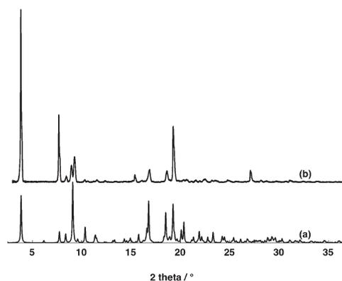
Fig. 9 Simulated (a) and observed (b) PXRD powder patterns for compound  $[7^{4-}\text{-}(A^{2+})_2]$ . Discrepancies in peak intensity are due to the preferential orientation of the microcrystalline powder.
